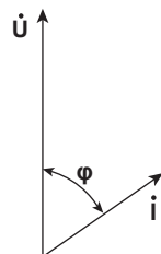
When the current lags the voltage
