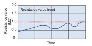
With this functionality, even inexperienced engineers can determine when adhesion occurs. Periodic maintenance is not necessary, as maintenance is only needed when impedance reaches the threshold level.
