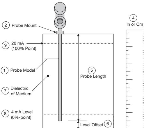
NOTE: A small transition zone (0–6") may exist at the top and bottom of the probe. See Specifications, Section 3.6.
