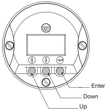
The ECLIPSE transmitter has an optional liquid crystal display (LCD) capable of showing two lines of 8 characters each. Transmitter measurements and configuration menu screens are shown on the LCD.
