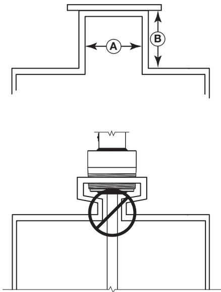
2. Ratio of Diameter: Length (A:B) is 1:1 or greater; any ratio <1:1 (e.g., a 2" x 6" nozzle = 1:3) may require a Blocking Distance and/or DIELECTRIC adjustment (see Section 2.6.5.2 Measurement Type: Level and Volume).
