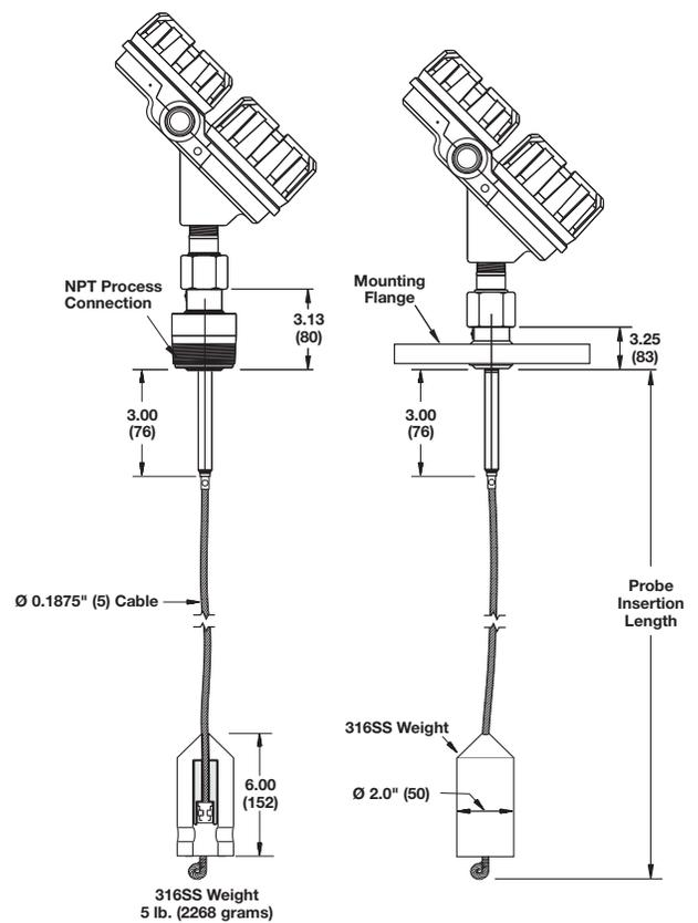
**Eclipse® with 7x2 Bulk Solids Flexible Probe
