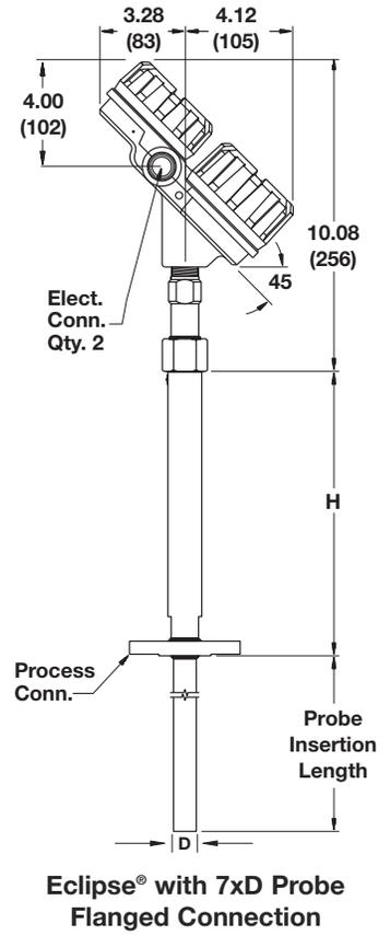
Eclipse® with 7xD Probe Flanged Connection
