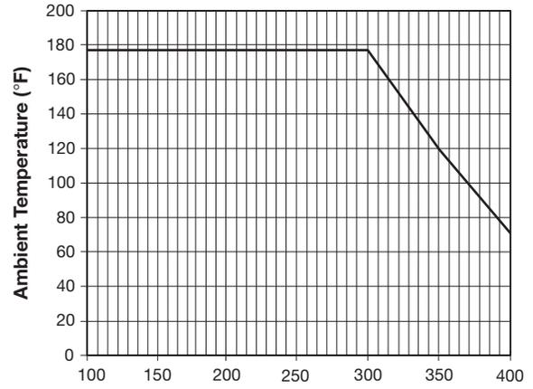
Ambient Temperature vs Process Temperature
