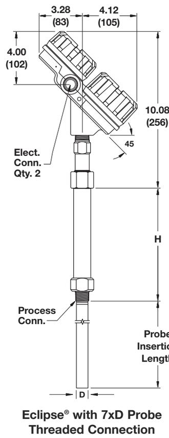
Eclipse® with 7xD Probe Threaded Connection
