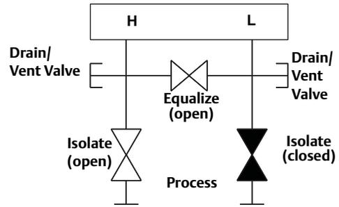
3. After zeroing the transmitter, close the equalizing valve.
