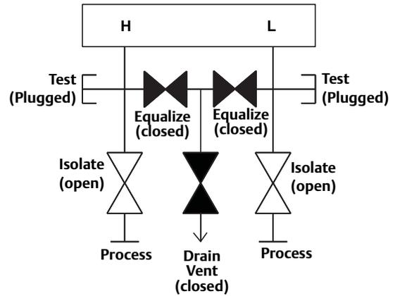
1. To zero the Rosemount 2051, first close the block valve on the low pressure (downstream) side of the transmitter.
