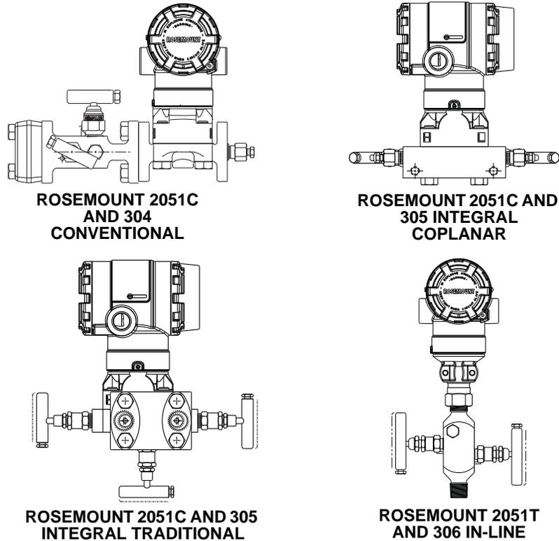
The 304 conventional manifold combines a traditional flange and manifold that can be mounted to most primary elements.
