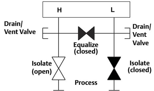
4. Open the block valve on the low pressure side of the transmitter to return the transmitter to service.
