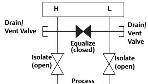
1. To zero the Rosemount 2051, close the block valve to the low pressure (downstream) side of the transmitter first.
