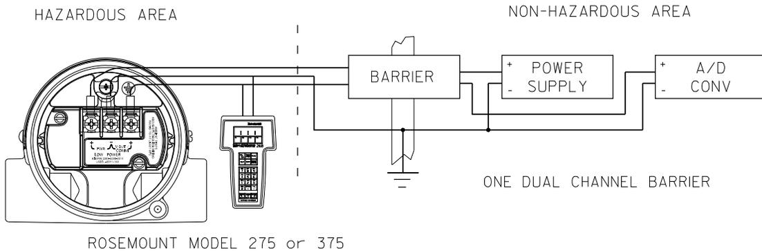
APPROVED FOR CLASS I, DIVISION I, GROUPS A,B,C,D WHEN USED IN CIRCUIT WITH TWO CSA APPROVED SINGLE CHANNEL SAFETY BARRIERS, ONE WITH APPROVED SAFETY PARAMETERS OF 28 VOLTS OR LESS AND 300 OHMS OR MORE IN +PWR LINE, AND ONE WITH APPROVED SAFETY PARAMETERS OF 10 VOLTS OR LESS AND 47 OHMS OR MORE IN Vout+ LINE, OR ONE CSA APPROVED DUAL CHANNEL SAFETY BARRIER WITH IDENTICAL APPROVED SAFETY PARAMETERS CONNECTED IN LIKE MANNER, AS ABOVE.
