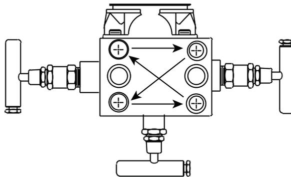
3. If the PTFE sensor module o-rings have been replaced, the flange bolts should be re-tightened after installation to compensate for cold flow of the o-rings.
