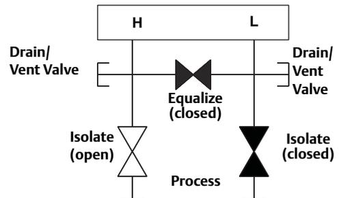
2. Open the center (equalize) valve to equalize the pressure on both sides of the transmitter. The manifold valves are now in the proper configuration for zeroing the transmitter.
