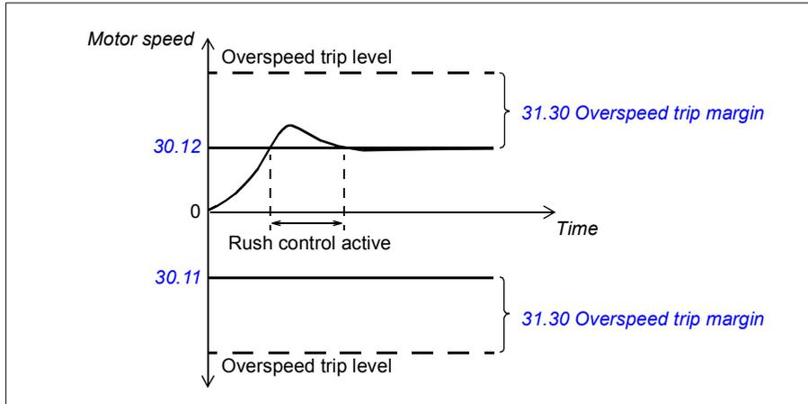
The function is based on a PI controller. The program sets the proportional gain to 10.0 and integration time to 2.0 s.
