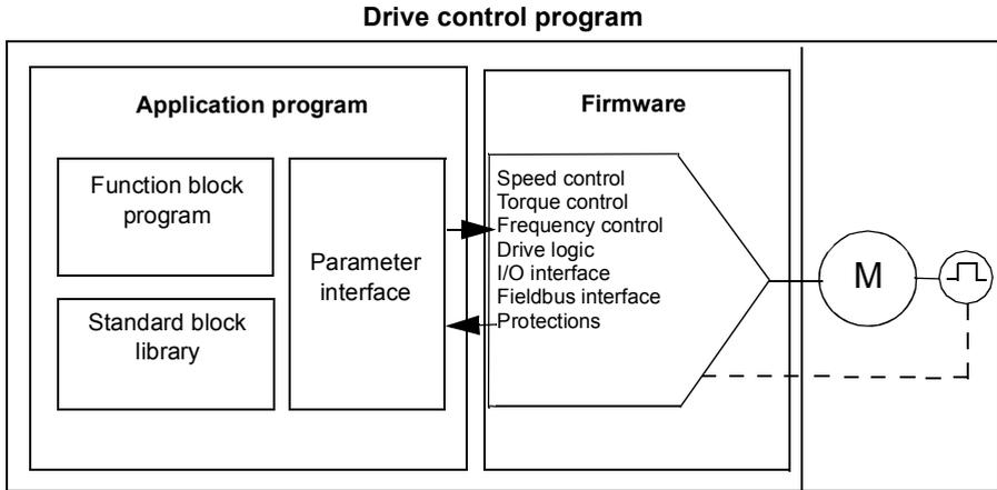
The firmware program performs the main control functions, including speed, torque and frequency control, drive logic (start/stop), I/O, feedback, communication and protection functions. Firmware functions are configured and programmed with parameters, and can be extended by application programming
