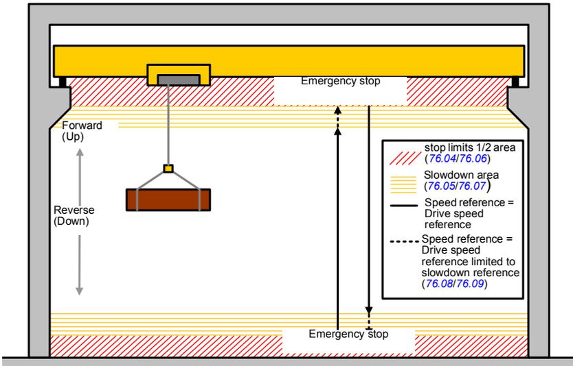
The crane slowdown function uses Limit to limit trigger type Level low (76.03) and has two modes:
