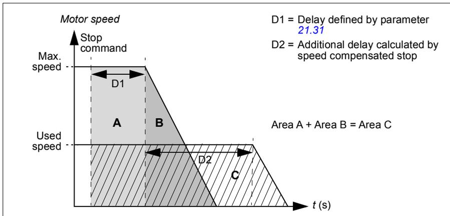
Speed compensation does not take into account shape times (parameters [23.32 Shape time 1](#) and [23.33 Shape time 2](#)). Positive shape times lengthen the distance traveled.
