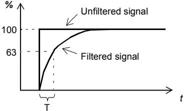
$O = I \times (1 - e^{-t/T})$ <p>I = filter input (step)<br/>O = filter output<br/>t = time<br/>T = filter time constant</p>                                                                                                                                                                                                                   | 0.100 s            |
