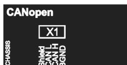
**Note:** When taking the CANopen module into use, it is recommended that the cord is not connected during the first start. This is to avoid disturbing the CAN bus when the drive attempts to recognize the attached module.
