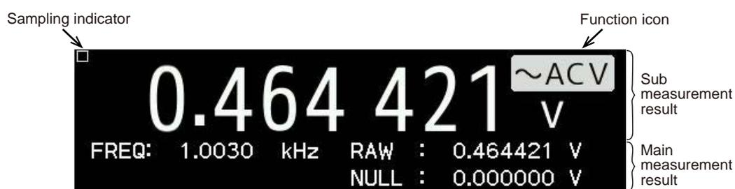
Figure 2.11(b) Example of NUMERIC display (FONT: NORMAL)
