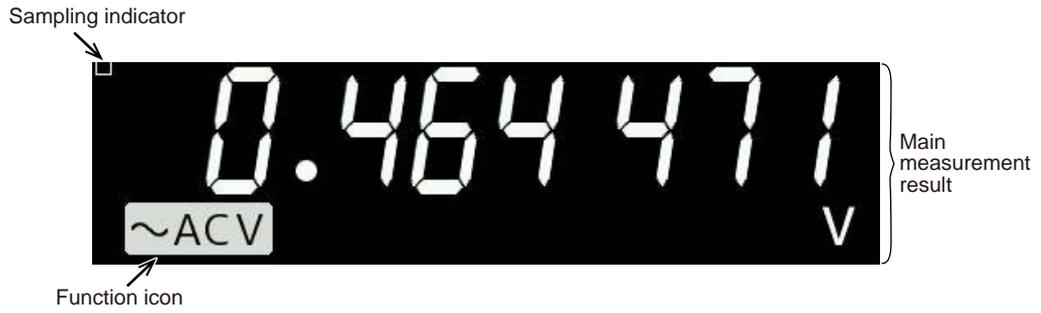
Figure 2.11(c) Example of NUMERIC display (FONT :7SEG)
