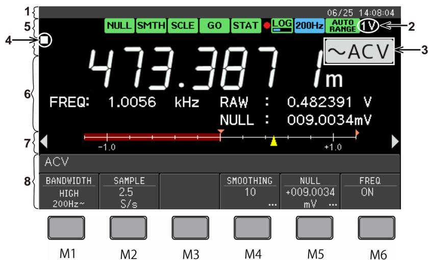
Figure 2.8(a) Example1 (PRIMARY: NUMERIC, SECONDARY: ANALOG METER)
