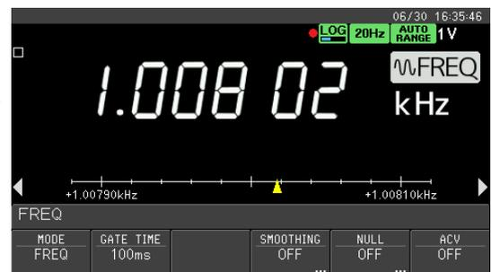
Figure 3.6(b) Frequency measurement (FREQ) screen
