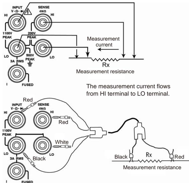
Connection method when using 4-terminal resistance measurement cable
