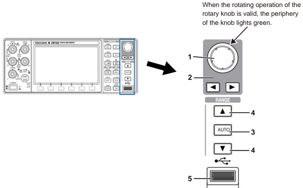
Figure 2.6 Rotary knob & RANGE switching part
