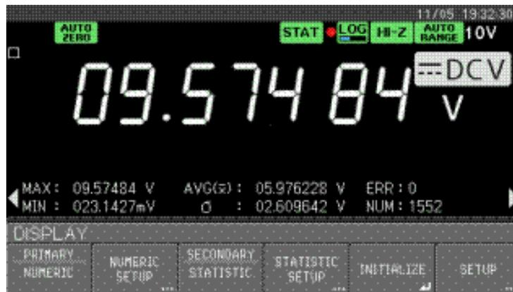
Figure 2.19 Example of STATISTIC calculation result display
