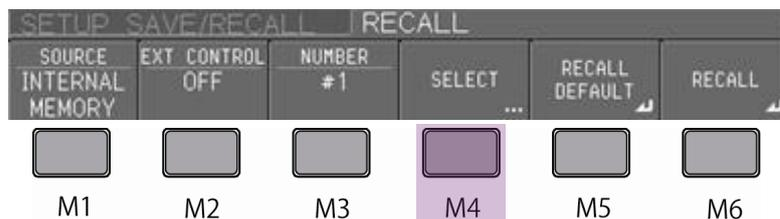
In 1) and 2) above, pressing M4 displays the summary of settings on the SETUP SUMMARY screen (the following is an example of #1) of the internal memory specified by the cursor.
