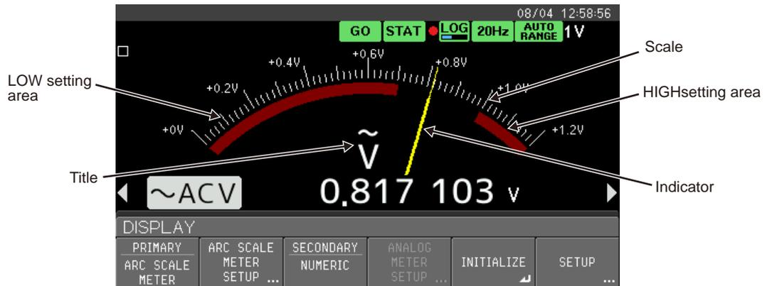
**Figure 2.15 Display example of ARC SCALE METER (NUMERIC)**
