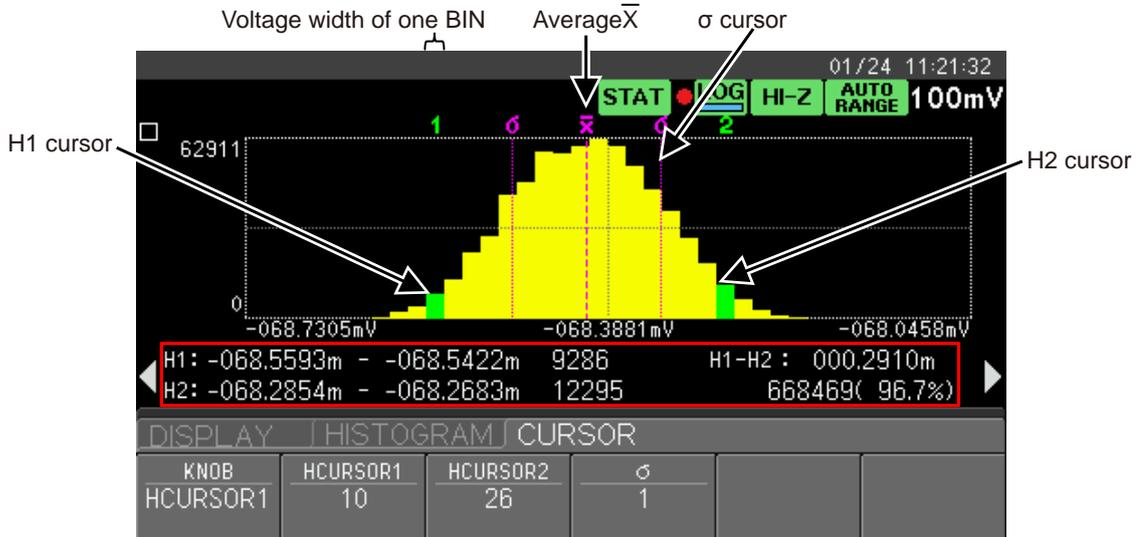
The histogram chart displays the frequency distribution of the entire measurement and is displayed as a bar graph as shown in the above figure. Each bar is called a bin. Each bin has a width. The width is voltage for voltage measurement and current for current measurement. The above figure is an example of a histogram chart display for DCV measurement.
