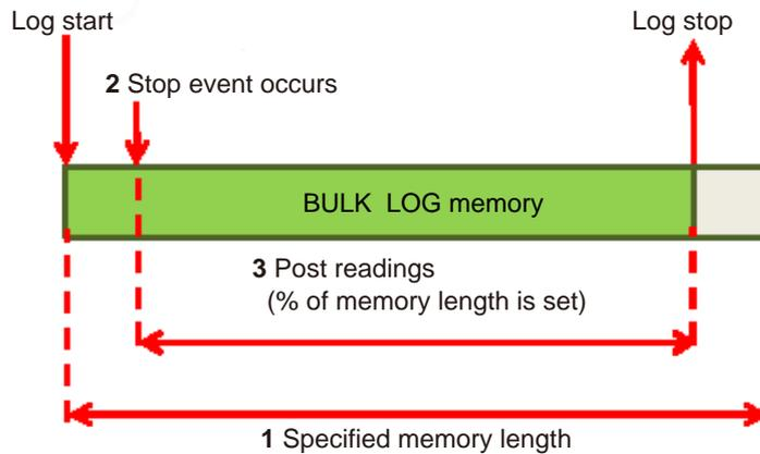
Press START LOG to start BULK mode measurement. The screen changes to BULK mode measurement (below), and measurement starts. (However, it is not possible to begin while continuously writing to the USB memory with the VALUE TO USB function.)
