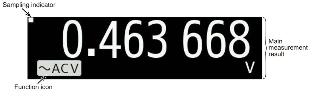
Figure 2.11(d) Example of NUMERIC display (FONT :NORMAL)
