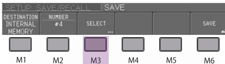
Pressing M3 displays the summary of settings on the SETUP SUMMARY screen (the following is an example of #4) of the internal memory specified by the cursor. See “Items and settings on SAVE (storage: internal memory) setting menu” below.
