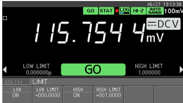
Figure 2.18 Example of LIMIT calculation result display
