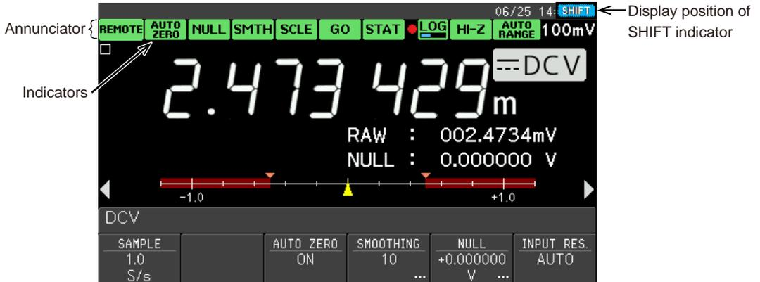
Figure 2.9 Example of annunciator and indicators
