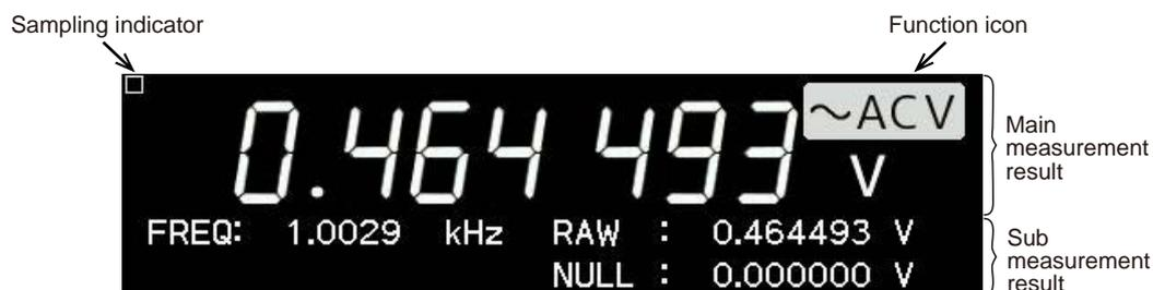
Figure 2.11(a) Example of NUMERIC display (FONT: 7SEG)
