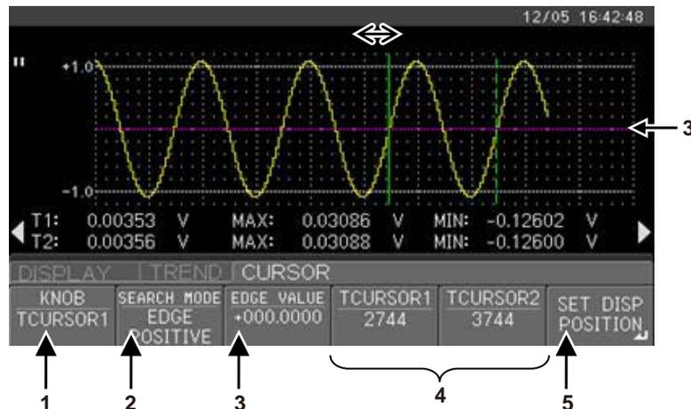
The measurement example shows the voltage, maximum (MAX), and minimum (MIN) values at the address specified by the T1 cursor (green solid line).
