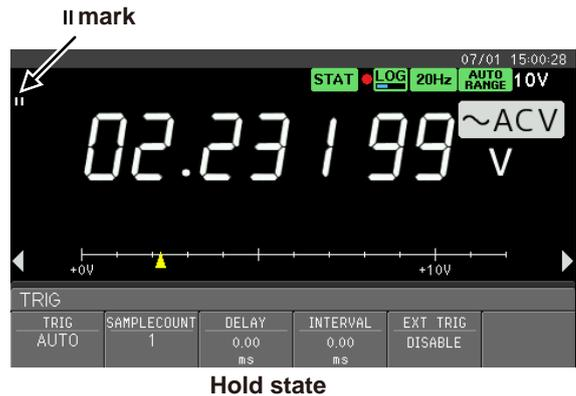
In addition to triggers using [HOLD/TRIG], the instrument can receive external triggers through the TRIG IN terminal on the rear panel and remote triggers from a remote control. (For the setting procedure, see 4.4.2.)
