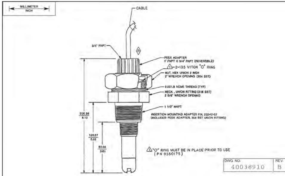
Figure 2-6: VP 8 Cable, Rosemount 389VP Sensor End
