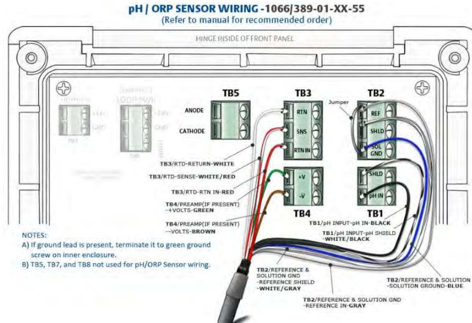
Figure 2-10: Rosemount 389-01-xx-55 Wiring to Rosemount 5091 Transmitter
