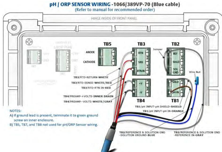
Figure 2-13: Rosemount 389VP Wiring to Rosemount 5081 Transmitter
