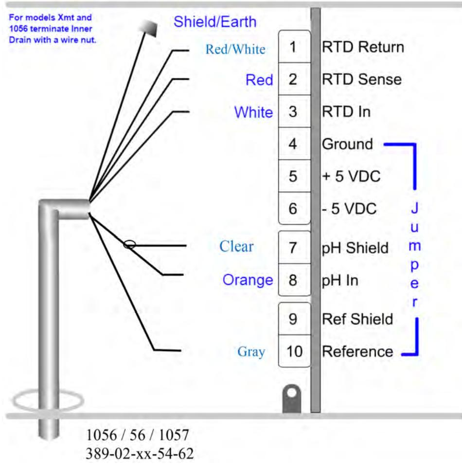
Figure 2-18: Rosemount 389-02-xx-54-62 Wiring to Rosemount 1066 Transmitter
