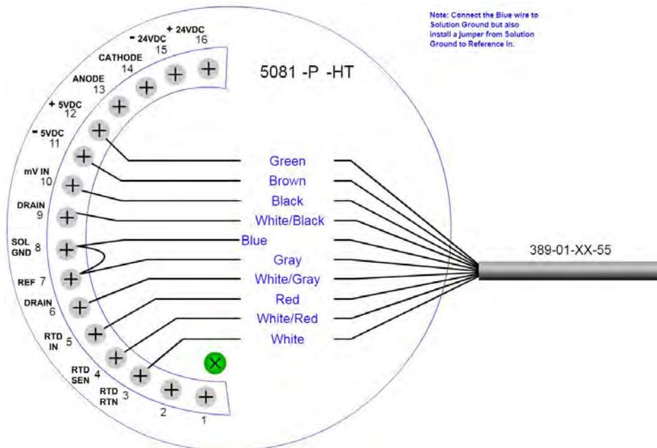
**Figure 2-11: Rosemount 389VP Wiring to Rosemount 1056, 1057, and 56 Transmitters**
