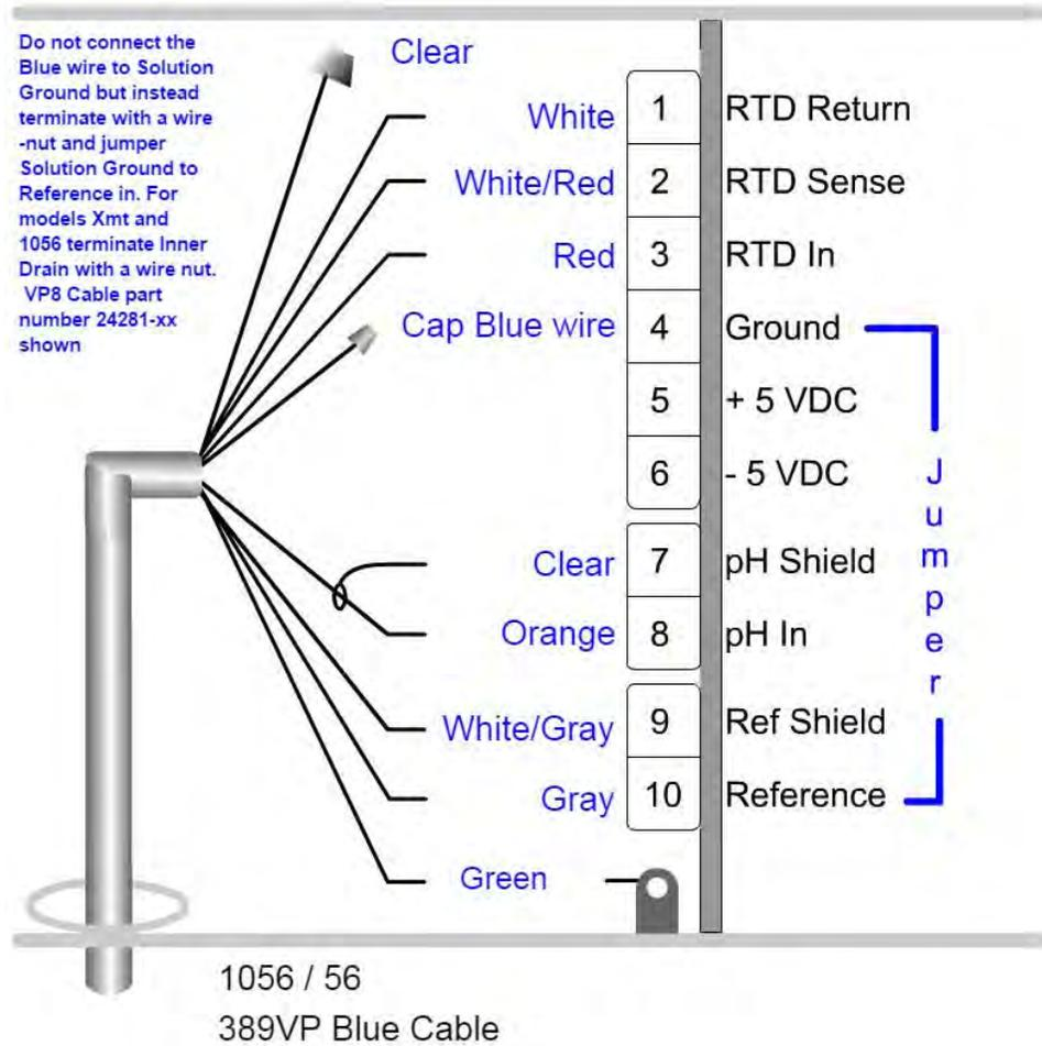
Figure 2-12: Rosemount 389VP Wiring to Rosemount 1066 Transmitter
