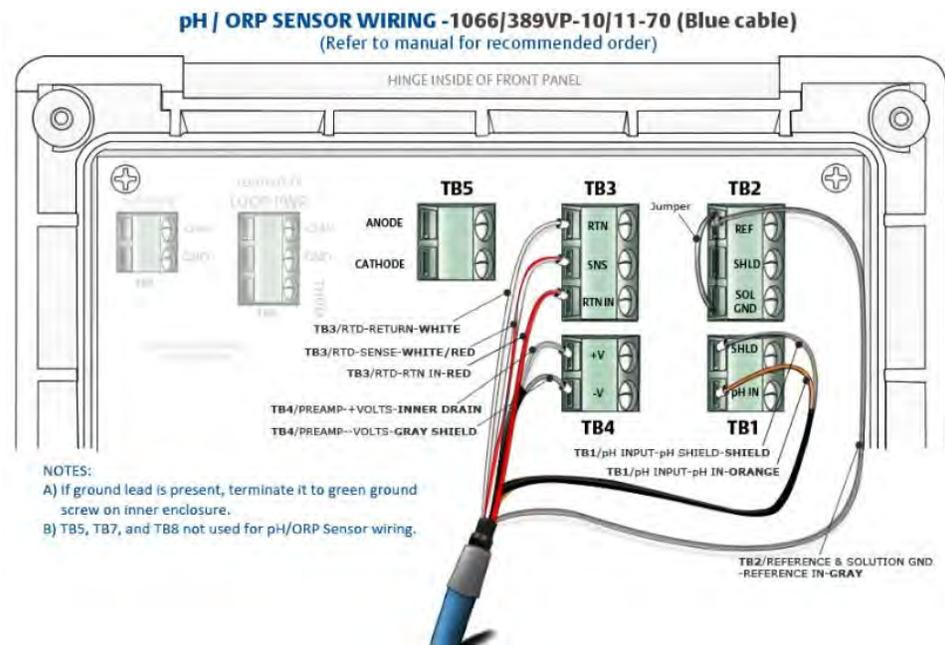
**Figure 2-16: Rosemount 389VP-xx-55-70 Wiring to Rosemount 5081 Transmitter**
