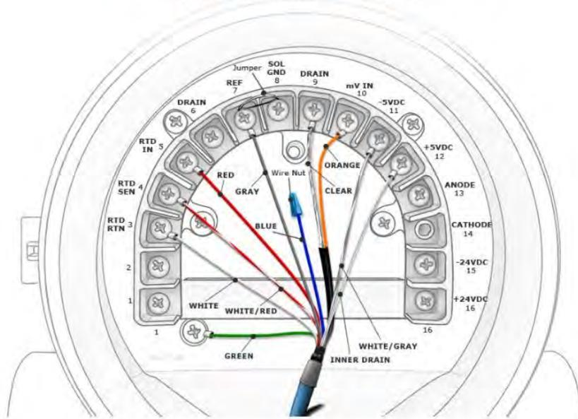
**Figure 2-17: Rosemount 389-02-xx-54-62 Wiring to Rosemount 1056, 56, and 1057 Transmitters**
