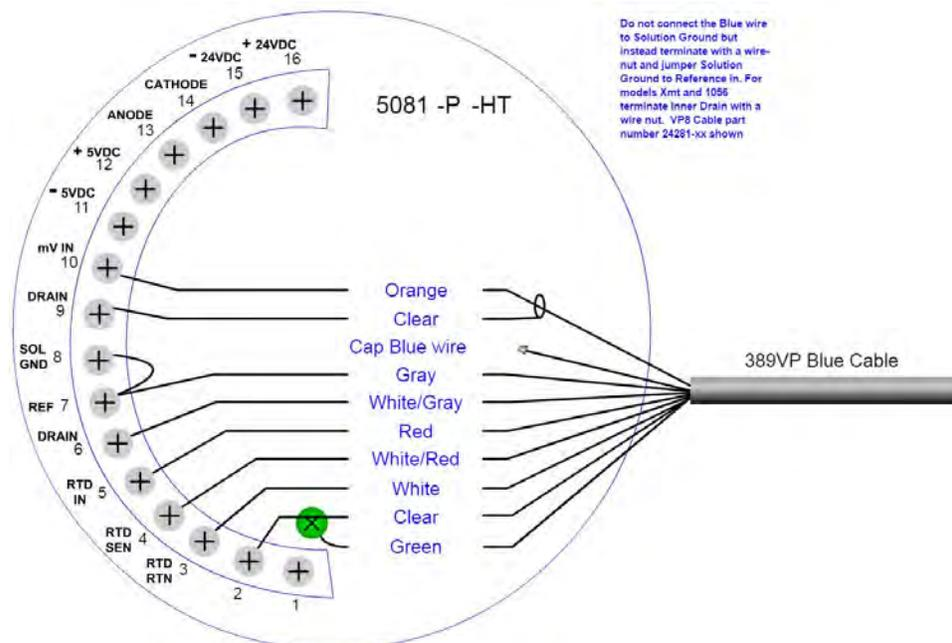
**Figure 2-14: Rosemount 389VP-xx-55-70 Wiring to Rosemount 1056, 1057, and 56 Transmitters**
