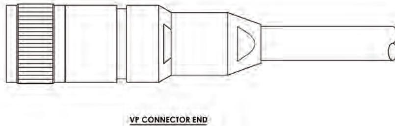
**Figure 2-7: VP8 Cable, Instrument End**
