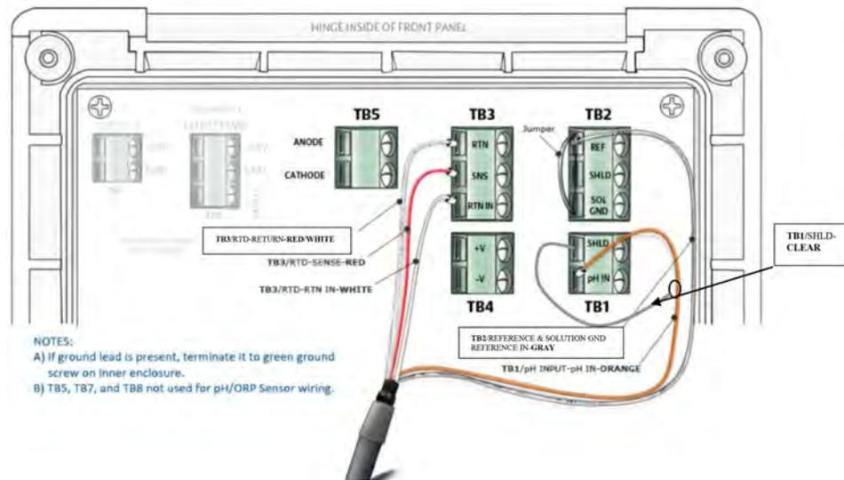
Figure 2-19: Rosemount 389-02-xx-54-62 Wiring to Rosemount 5081 Transmitter
