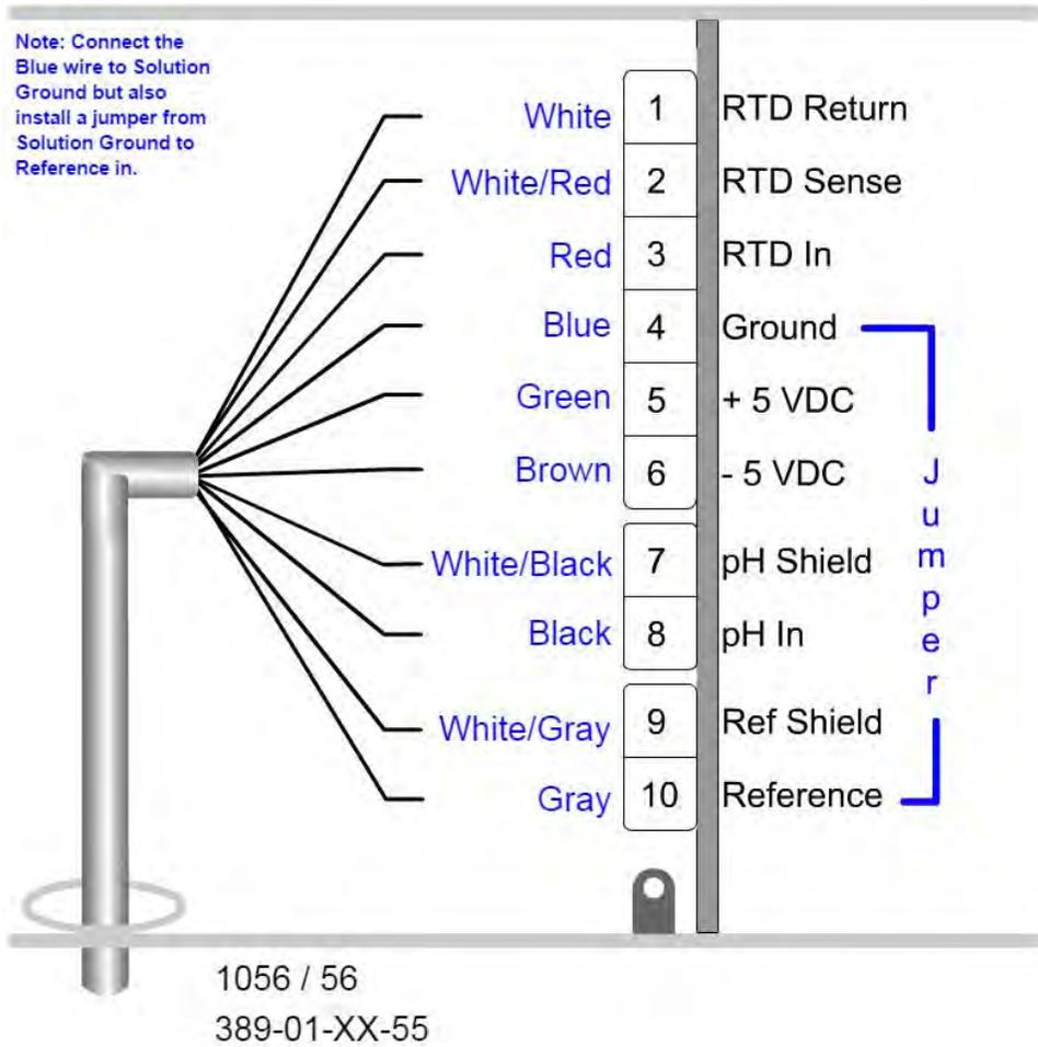
Figure 2-9: Rosemount 389-01-xx-55 Wiring to Rosemount 1066 Transmitter
