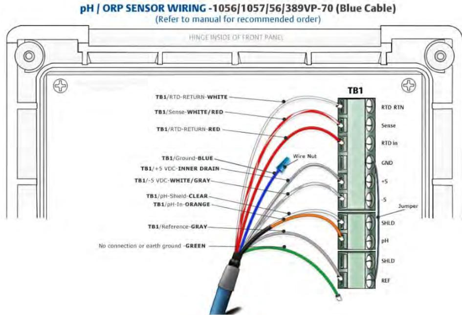
**Figure 2-15: Rosemount 389VP-xx-55-70 Wiring to Rosemount 1066 Transmitter**
