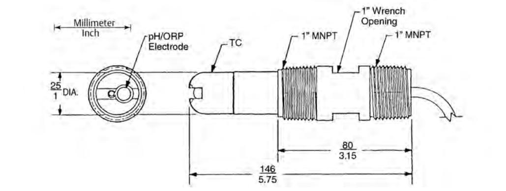
Figure 2-2: Rosemount 389VP Sensor dimensional drawing
