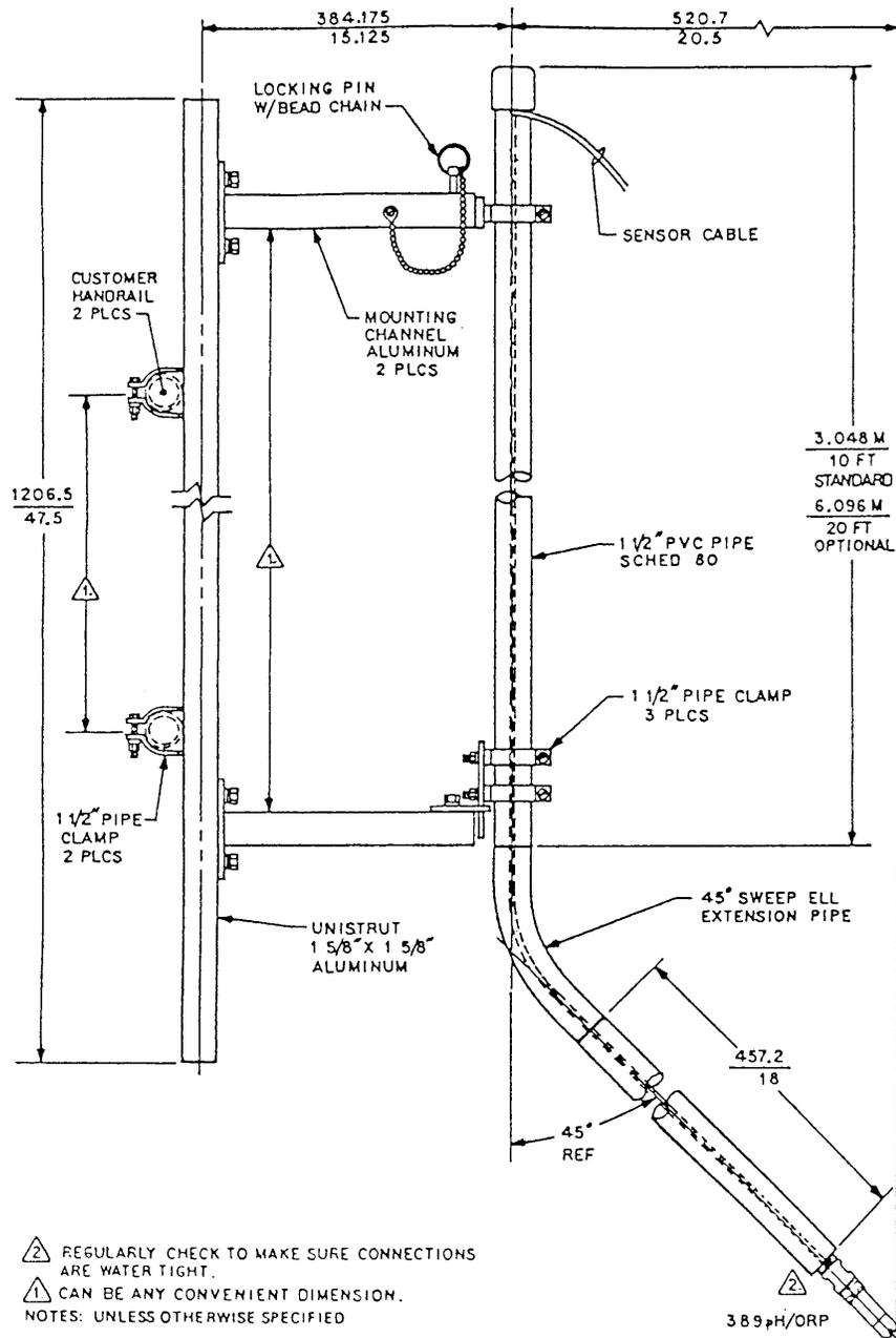
4. Run the sensor cable through a protective conduit for isolation from electrical interference or physical abuse from the process.
