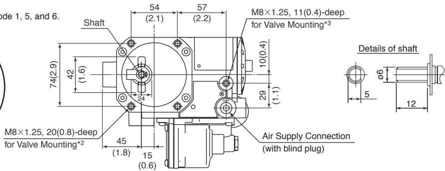
\*2: Attached with 4 mounting bolts (M8, 25 mm) and spring washers (applicable 3 to 6 mm thick brackets).
