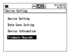
2. Use the ▲ or ▼ key to select Firmware Upgrade and press the ENTER key.
