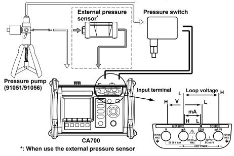
The CA700 can calibrate mechanical pressure switches. It cannot be used to calibrate open-collector contact, voltage output, or current output pressure switches.
