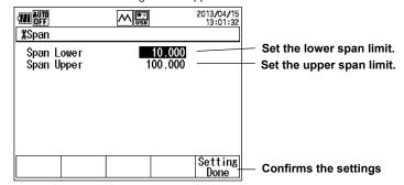
38. Press the d or ► key to move to the digit you want to change, press the d or key to set the number.
