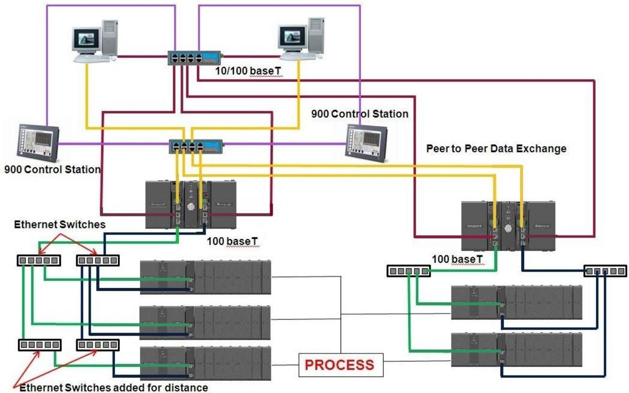
Figure 7 - Multiple Systems / Multiple Racks
