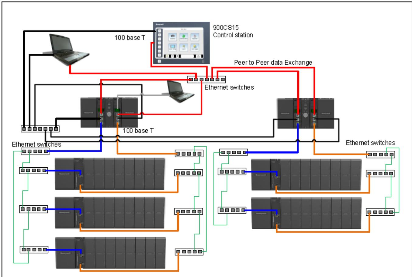
**Figure 6 MULTIPLE PROCESS/MULTIPLE RACKS - RED NETWORKS (RING TOPOLOGY)**
