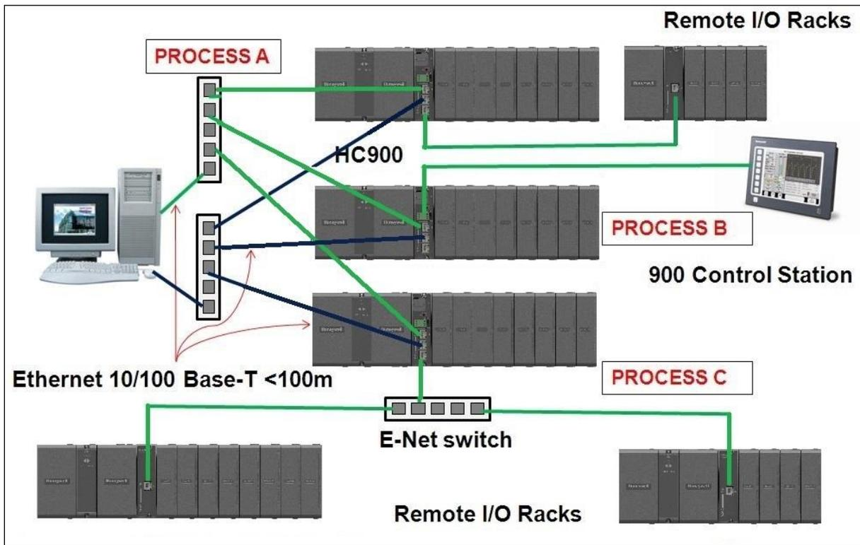
Figure 5 - MULTIPLE PROCESS/MULTIPLE RACKS – RED NETWORKS (STAR TOPOLOGY)
