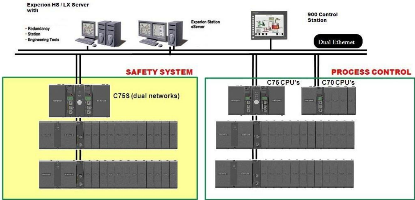
**Figure 8 - Safety and Non-Safety in Separate Systems**
