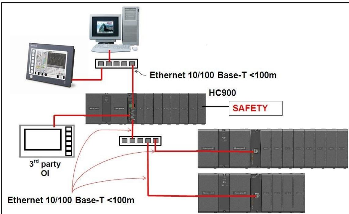
Figure 3 - SINGLE PROCESS/MULTIPLE REMOTE RACKS- SAFETY
