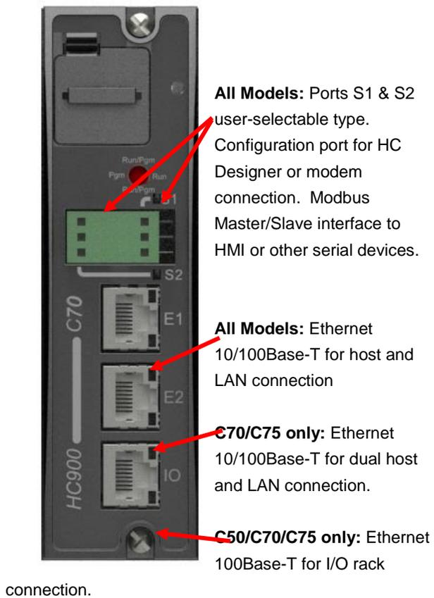
**Figure 9 - Communication ports**
