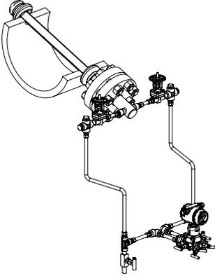
**Figure 11. Vertical Steam and Liquid**
