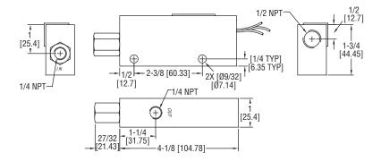
The SERIES P1 Brass Flow Switches utilizes a piston-type design for accurate detection of excessive or insufficient liquid flow rates. The switches have preset actuation points from 0.10 to 1.5 GPM for liquid flow.
