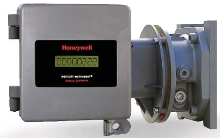
This direct-mount electronic volume corrector is available for most popular rotary gas meters. The internal temperature probe and independent Redundant Electronic Index (REI) improve the precision and reliability. The Mini-Max Rotary Corrector easily adaptes to Dresser LMMA & B3, Romet and Elster American Meter\* B & C-body rotary meters.
