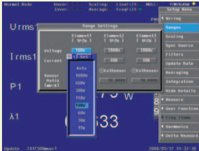
Example of voltage range setting
