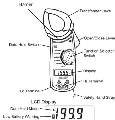
Barrier: It is a part providing protection against electrical shock and ensuring the minimum required air and creep age distances.
