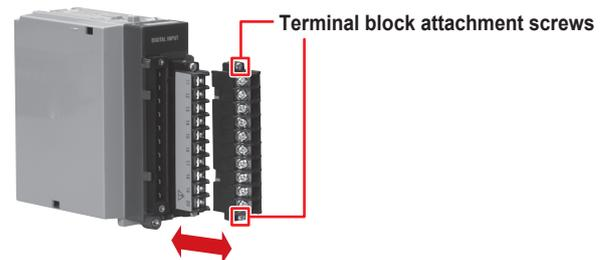
Recommended torque for tightening the terminal block attachment screws: 0.1 N·m
