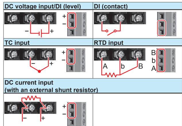
\* Be careful because the DI wiring is different between level and contact.
