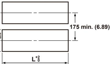
**Side-by side mounting (vertically; max. 3 units)**
