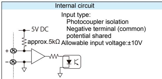
Note: Do not apply voltage outside the allowable input voltage range across input terminals. Doing so can cause a malfunction.
