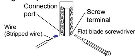
First, loosen the screw at the front using a flat-blade screwdriver. Insert the input signal wire into the slit on the left side of the terminal block, and fasten the screw at the front.
