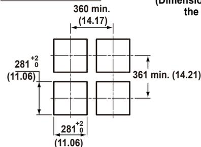
(Dimensions after attaching the mounting bracket)
