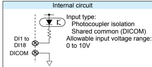
Note: Do not apply voltage outside the allowable input voltage range across input terminals. Doing so can cause a malfunction.
