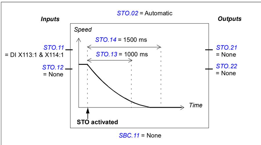
**Example 2 (with an encoder):** The figure below shows an example of a simple STO function set-up when an encoder is used. Configure the safety encoder interface first (see section [Configuring the safety encoder interface](#) on page 277).
