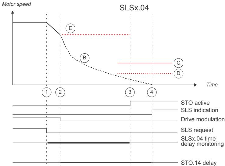
1. SLS request is activated (SLSx.11 SLS1 input A = DI X113:2 & X114:2). SLS time delay monitoring is started (SLSx.04 SLS time delay = 2000 ms). Deceleration to SLS limit speed is started (drive parameter 23.13 Deceleration time 1).
