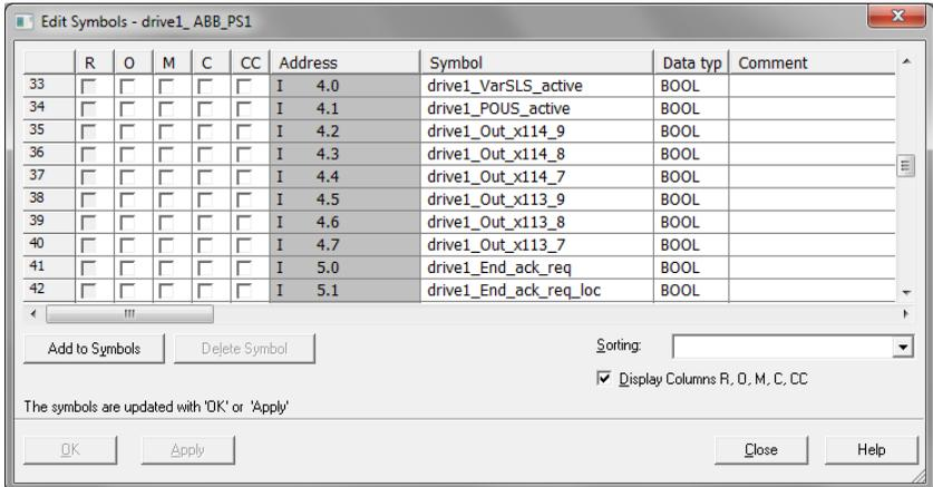
**Note:** In PROFINET communication, the bits of each octet are sent the most significant bit first. Therefore, the bits of every octet in the PROFINET message are in reversed order compared to the bits shown in the figure. For example, the first bit that is sent in the PROFINET message is the 7th bit of the first octet (I 0.7).
