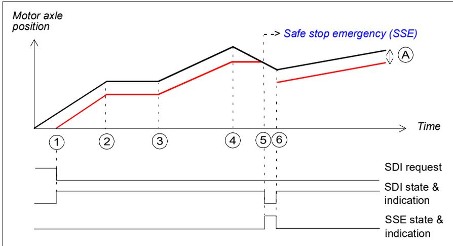
A SDI tolerance limit degree (parameter [SDI.14](#)): The motor axle cannot move to the forbidden direction more than defined with this parameter.
