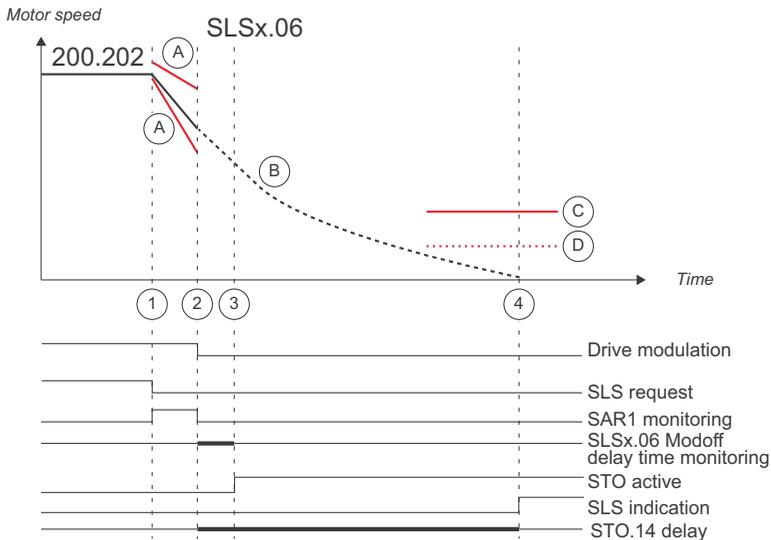
1. SLS request is activated (SLSx.11 SLS1 input A = DI X113:2 & X114:2). SLS ramp monitoring is activated (SAR1). Parameter 200.202 SAR speed scaling (= 1500 rpm) is used as a reference point in ramp time calculations. Deceleration towards the SLS limit speed is started according to SAR1 parameters:
