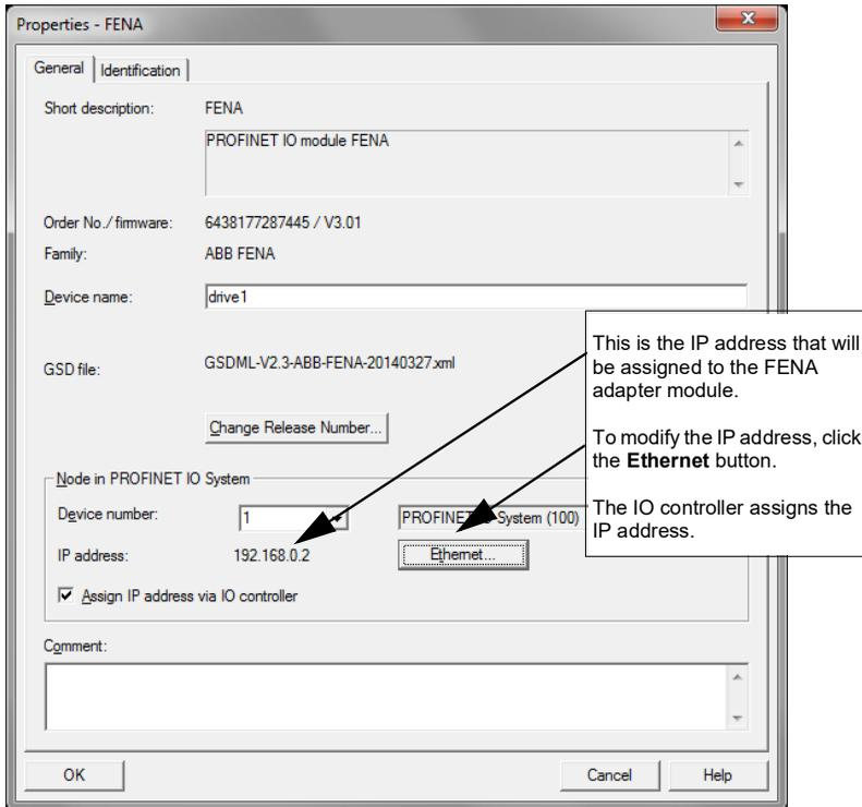
**Note:** Do not change the IP address assigned here. Use the same IP address for the FENA adapter module also in other tools (eg, the Drive composer pro PC tool) which you use to connect to the drive.
