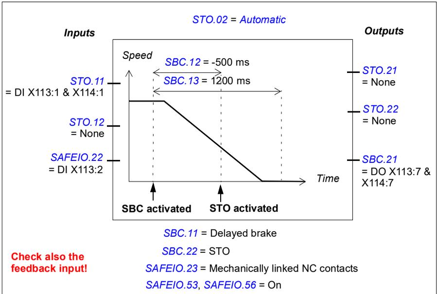
**Example 2 (with an encoder):** The figure below shows an example of the SBC before the STO set-up when an encoder is used. Configure the safety encoder interface first (see section [Configuring the safety encoder interface](#) on page 277).
