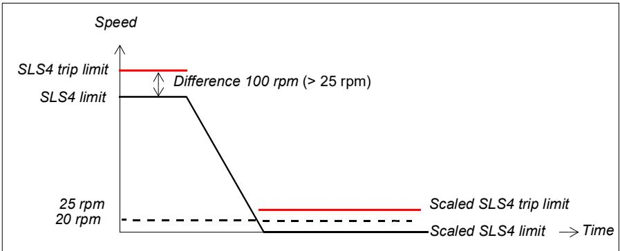
**Example 3 (with encoder):** The original SLS4 and SLS4 trip limits are: 100 and 110 rpm. The scaling value is 10%. The zero speed value is 10 rpm.
