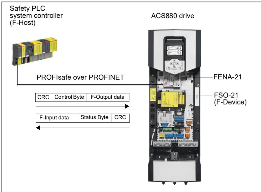
The FSO-21 safety functions module and the FENA-21 Ethernet adapter module are installed on the ACS880 drive. The safety PLC is connected to the FENA module, which communicates with the FSO module. The safety PLC activates safety functions via the PROFIsafe communication bus. The user can also activate safety functions from an I/O device (for example, an emergency stop button) which is connected to the FSO module.
