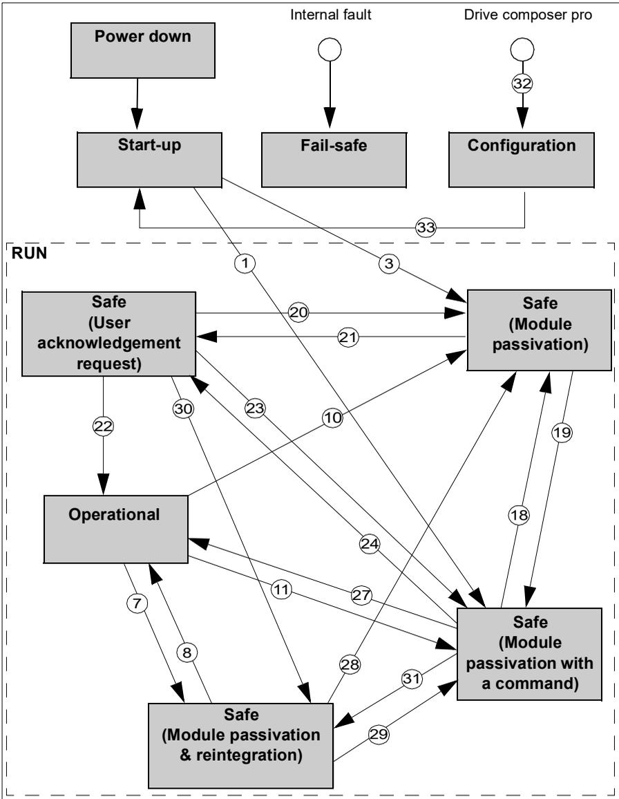
**Note:** It is possible to go to the Configuration mode from any other state when the drive is not modulating. From the Configuration mode, it is possible to go only to the Start-up mode.
