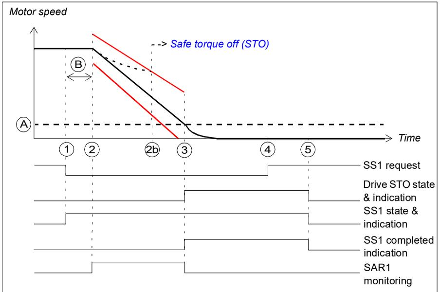
A Zero speed with encoder (parameter [FSOGEN.52](#)): Speed limit for activating the drive STO function. The safety function is completed, ramp monitoring is stopped and the SS1 completed indication (parameter [SS1.22](#)) goes on. The acknowledgment becomes allowed.
