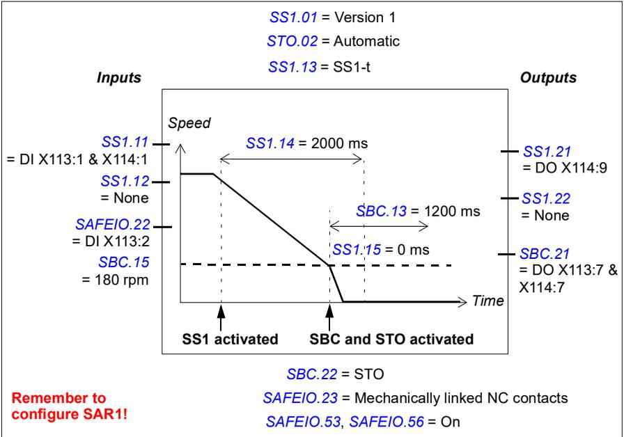
**Example 2:** The figure below shows an example of the SS1-r function with speed limit activated SBC set-up:
