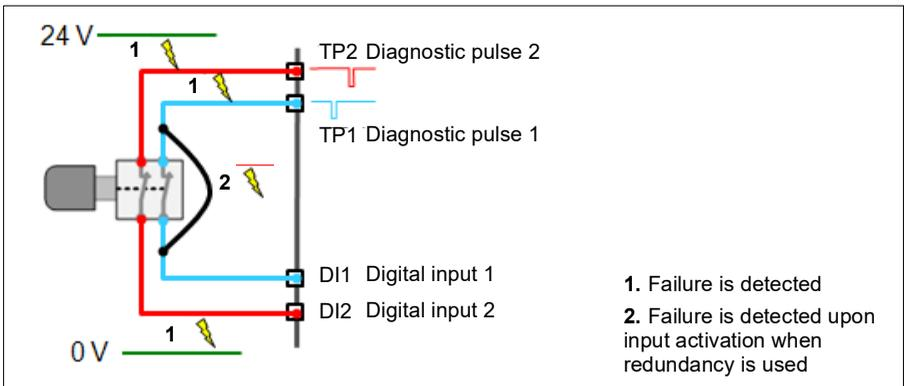
**Note:** If only one of the redundant inputs is activated upon a safety function request, the FSO module activates the safety function but it cannot be acknowledged before the failure has been repaired. To acknowledge the safety function, you must set both input channels down and up at the same time or, switch the power off and on.
