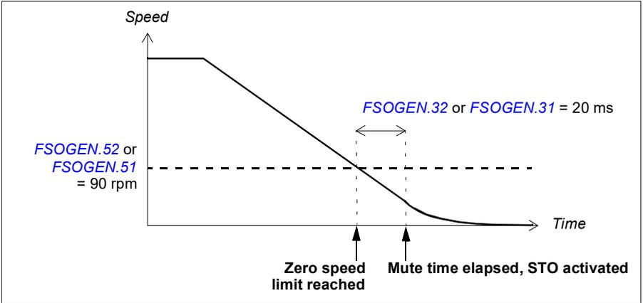
**Example 2:** Zero speed limit is reached in the SS1 function (and SSE with emergency ramp), a negative SBC delay (parameter *SBC.12 STO SBC delay*) is configured in the STO function:
