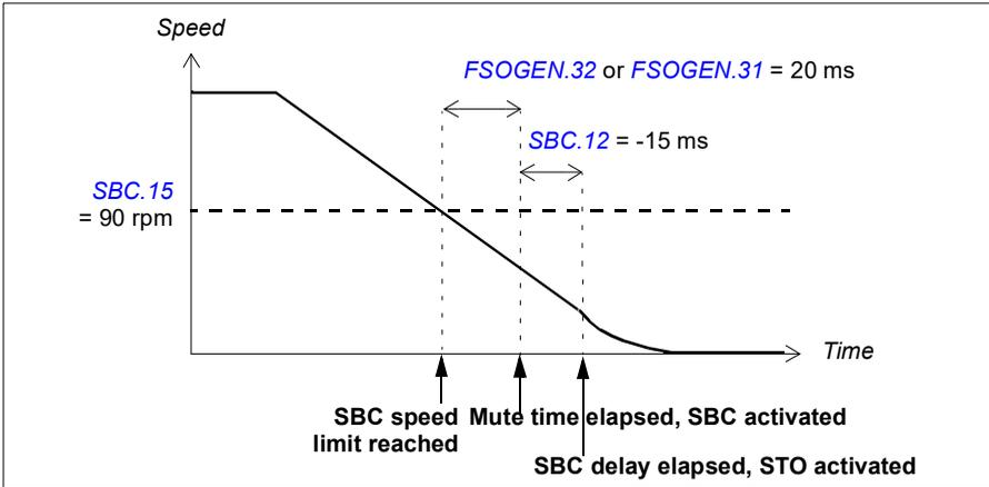
**Note:** If the SBC delay (parameter *SBC.12* *STO SBC delay*) is positive or zero (0 ms), the SBC and STO functions are activated at the same time.
