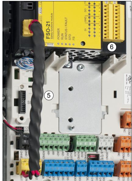
7. Connect the power supply wires to the FSO terminal X112. Use the tightening torque of 0.24 Nm (2.1 lbf-in) for the FSO terminals. Use proper cable strain relief. See also section [Power supply connection/cables](#) on page 255.
