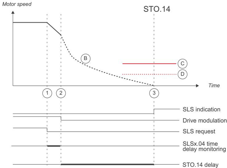
1. SLS request is activated (SLSx.11 SLS1 input A = DI X113:2 & X114:2). SLS time delay monitoring is started (SLSx.04 SLS time delay = 2000 ms). Deceleration to SLS limit speed is started (23.13 Deceleration time 1).
