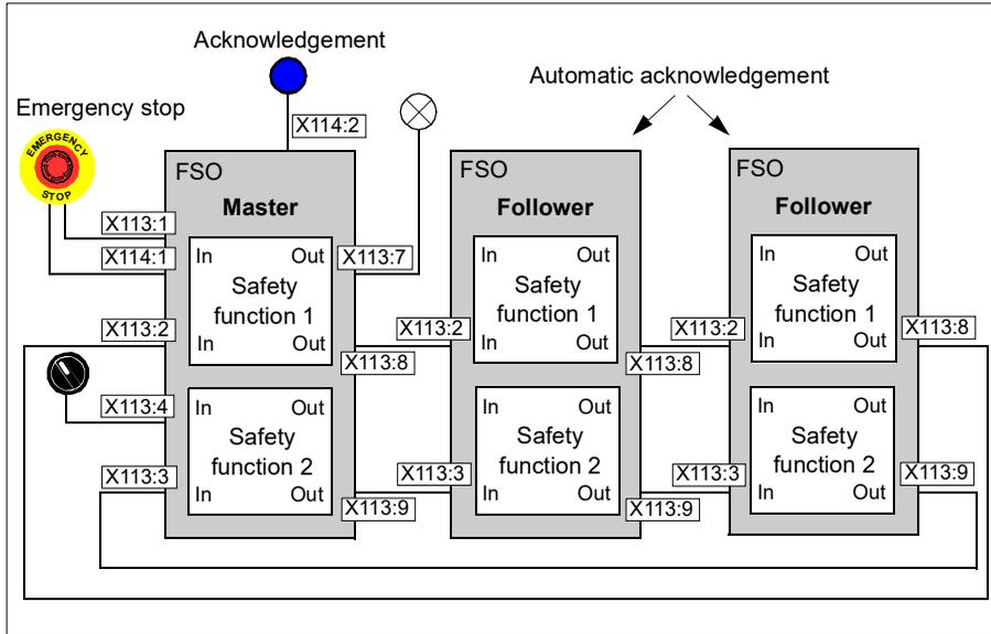
The inputs and outputs of the FSO module are defined as pairs. In this example, single input X113:2 is cascaded with single output X113:8. When Emergency stop (Safety function 1) is activated in the master FSO module (from redundant digital input X113:1&X114:1), it is also activated in the follower FSO modules. Safety function 2 is cascaded with single input X113:3 and single output X113:9.
