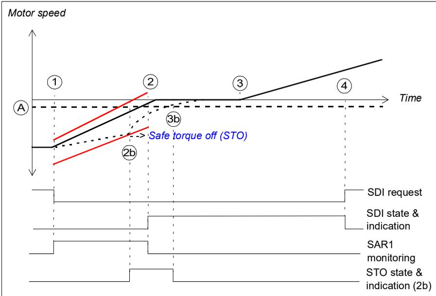
A Zero speed with encoder (parameter [FSOGEN.52](#)): Speed limit to define the motor as stopped. The safety function is completed and the STO completed indication (parameter [STO.22](#)) goes on. The STO acknowledgment becomes allowed.
