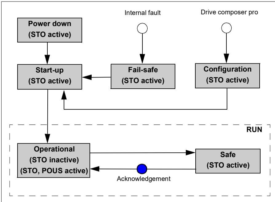
At power-up, the FSO goes into the Start-up mode; it performs start-up checks and, according to the configuration, enters the Operational state either automatically or after an acknowledgement request from the FSO I/O or from a safety PLC.
