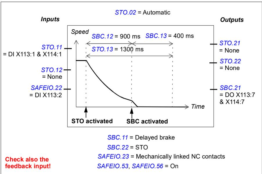
**Example 2 (with an encoder):** The figure below shows an example of the SBC after the STO function set-up when an encoder is used. Configure the safety encoder interface first (see section [Configuring the safety encoder interface](#) on page 277).
