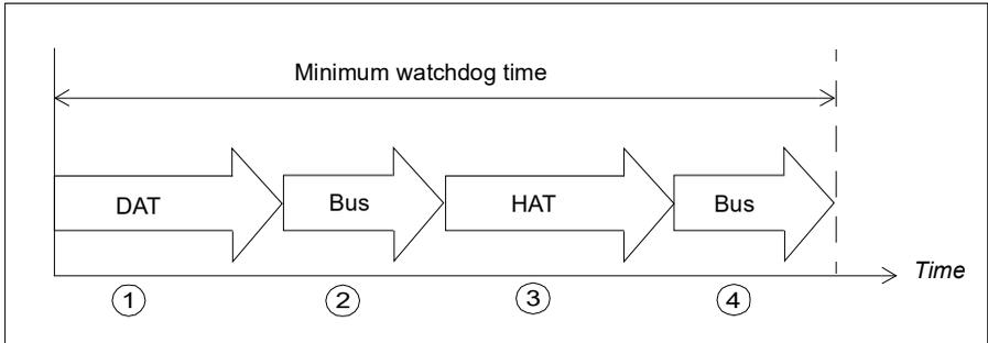
1. Device acknowledgement time (DAT) is the time it takes for the F-Device (such as the FSO module) to process an incoming PROFIsafe frame. DAT starts when the F-Device receives the PROFIsafe frame and ends when the F-Device has prepared a new PROFIsafe frame using the currently available process values.
