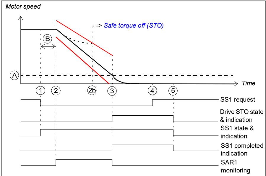
A Zero speed (parameter [FSOGEN.51](#)): Speed limit for activating the drive STO function. The safety function is completed and the SS1 completed indication (parameter [SS1.22](#)) goes on. The acknowledgment becomes allowed.
