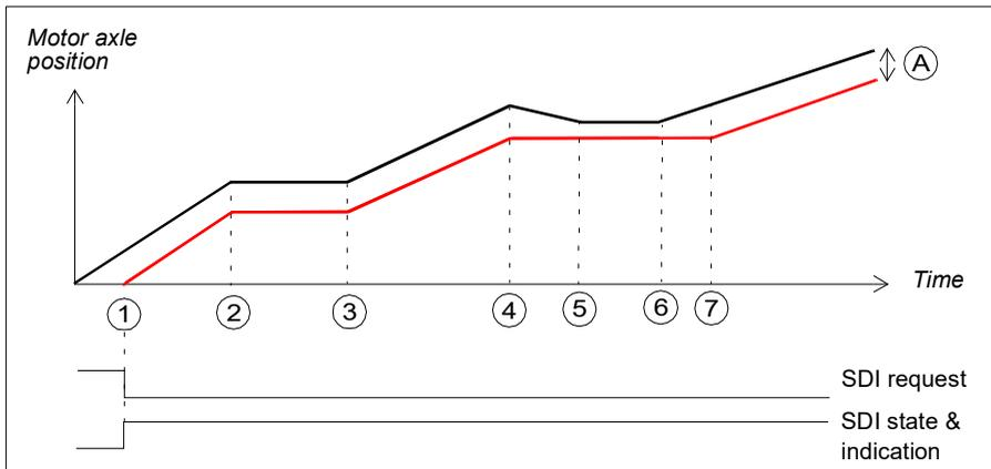
A SDI tolerance limit degree (parameter [SDI.14](#)): The motor axle cannot move to the forbidden direction more than defined with this parameter.
