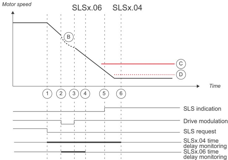
1. SLS request is activated (SLSx.11 SLS1 input A = DI X113:2 & X114:2). SLS time delay monitoring is started (SLSx.04 SLS time delay = 2000 ms). Deceleration to SLS limit speed is started (23.13 Deceleration time 1).
