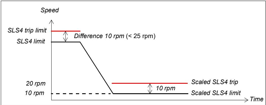
**Example 2 (no encoder):** The original SLS4 and SLS4 trip limits are: 1000 and 1100 rpm. The scaling value is 0%. The zero speed value is 20 rpm.
