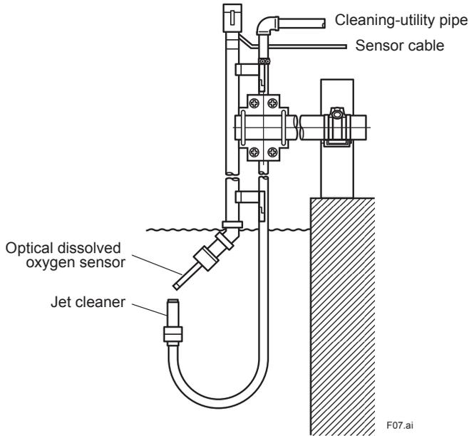
**Figure 2.3** Suspension of Optical Dissolved Oxygen Sensor Using DOX8HS Submersion Type Holder (with Jet Cleaner)
