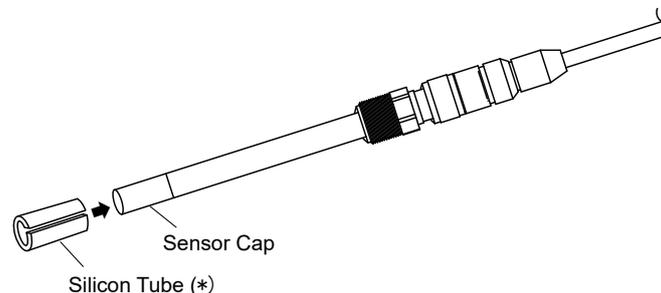
(\*): When you attach or detach the sensor cap, use an attached silicon tube and so forth.
