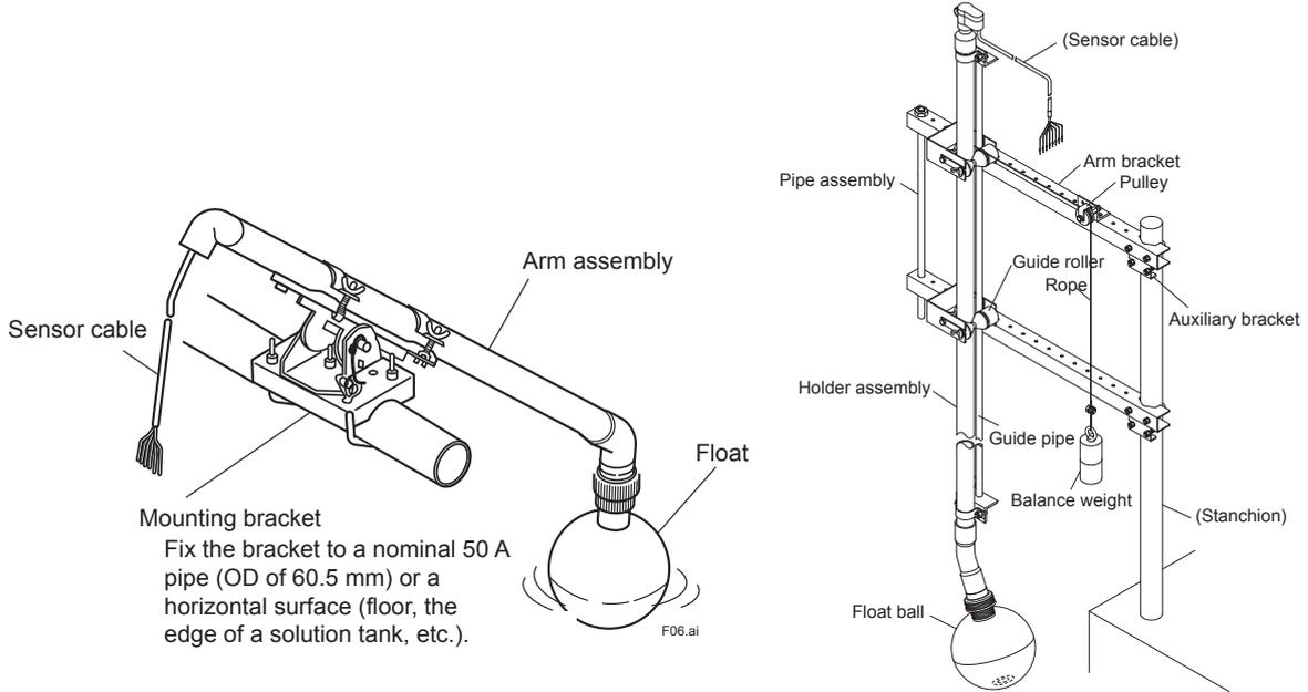
Figure 2.2 Suspension of Dissolved Oxygen Sensor Using PB350G Angled Floating Ball Holder
