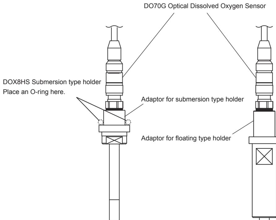
Figure 2.1 Assembling the Adaptor
