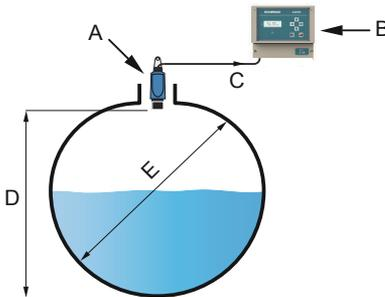
P013 = Full Volume of Ideal Cylindrical or Spherical Tank of Constant Diameter P014
