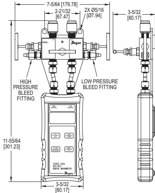
The **Series 490A-HKIT Hydronic Differential Pressure Meter Kit** features the 490A Hydronic Differential Pressure Manometer and all the necessary attachments and accessories to meet all your balancing, measuring, and pressure needs. The manometer featured in this kit is a versatile, handheld, battery operated manometer available in several ranges for positive or positive differential pressure measurement and can tolerate most liquid media compatible with 316L SS.
