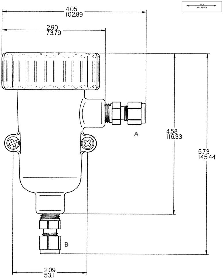
Inlet and outlet connections are stainless steel and take ¼-in. OD tubing. Flow cell is polycarbonate with ¼-in. FNPT fittings.
