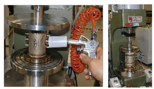
Testing with an Helium-leakage detector
