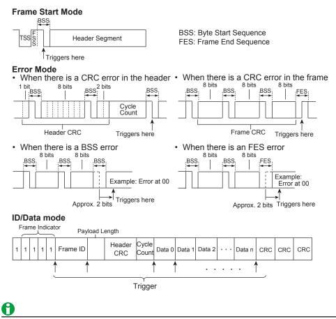
When the trigger mode is set to Error, the DLM2000 uses its internal sampling clock for sampling, so jitter equal to one period of the sampling clock arises. One period of the sampling clock is a period of time equal to 1/8 of the bit width at the specified bit rate. For example, when the bit rate is 5 Mbps, the jitter is 25 ns.
