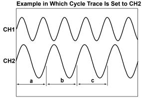
Measures the items in ranges a, b, and c, and calculates statistics on the items in the order a, b, and c. The items of other channels are also measured in ranges a, b, and c. If you select Own, the items are measured over each waveform's period.
