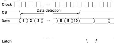
The latch signal specifies the time when data is compared. Trigger point
