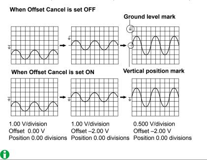
• The offset setting applies to all input coupling settings (AC, DC, DC50, and GND).
