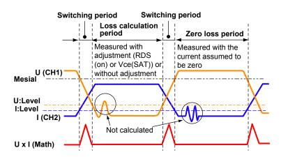
Loss calculation period: The period from the point where the voltage waveform goes below the U:Level
