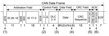
Positions (1) to (6) above are trigger points for the following conditions. (1) SOF
