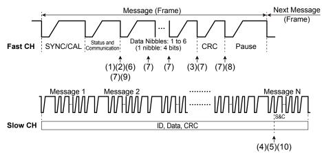
Positions (1) to (10) above are detected points for the following conditions.
