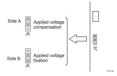
Figure 4.5 "Applied Voltage Compensation/Applied Voltage Fixation" Selection Jumper
