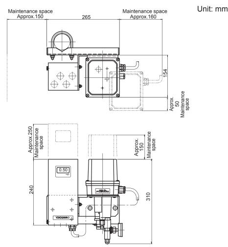
Figure 3.1 Maintenance Spaces for the FC500G Free Available Chlorine Analyzer
