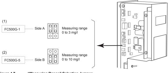
Figure 4.7 "Measuring Range" Selection Jumper
