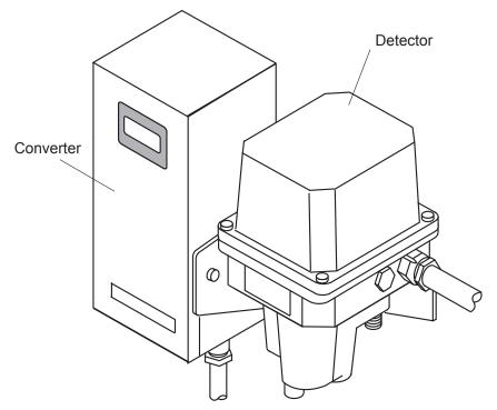
Figure 1.1 Appearance of Model FC500G Free Available Chlorine Analyzer
