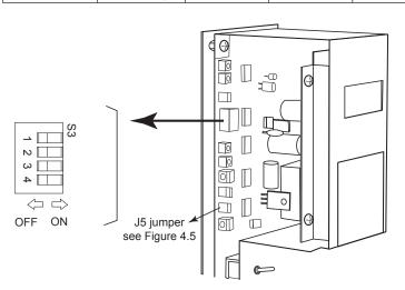
Figure 4.4 Measuring Range Setting Switch
