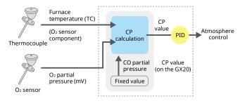
Electronic component firing/drying furnace temperature control, and recording of managed data
