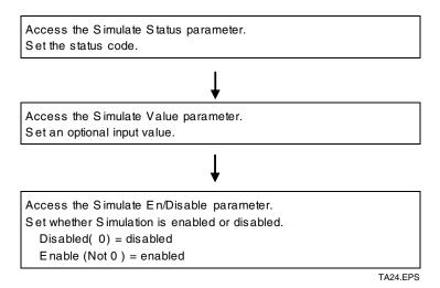
If simulation is enabled, AI block uses Simulate Status and Simulate Value as the input, and if disabled, the AI block uses Transducer Status and Transducer Value as input.
