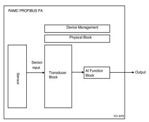
Figure 2.1 Logical Structure of Each Block
