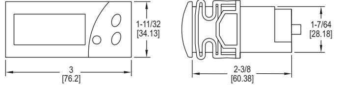
The affordable **Series TID** allows user to monitor temperature or a process value. Temperature ranges are available from -58 to 302°F using one of our PTC or NTC thermistors. Process values can be displayed from -999 to 999 counts using a 4-20 mA signal from one of our various transmitters. The process indicator has an adjustable span and zero on the 4-20 mA models.
