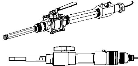
Top: 4909 SS Insertion/Removal Cell Assembly
