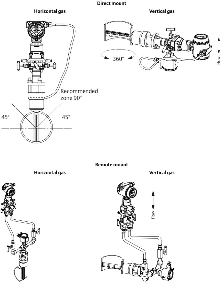
**Figure 6. Flowmeter Orientation for Steam**
