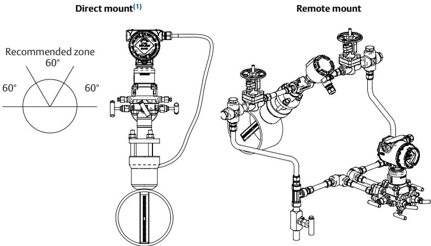
1. For wet steam, do not mount the flowmeter at the direct vertical position. Mounting at an angle will avoid measurement inaccuracy due to water running along the bottom of the pipe.
