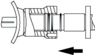
7. Tighten the nuts onto the studs:
