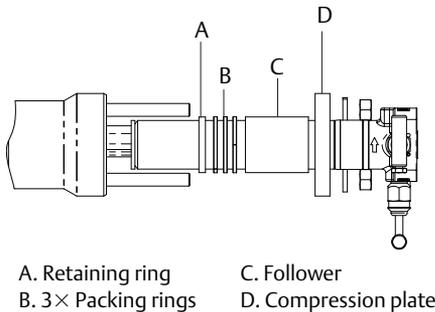
6. Push the packing ring into the Pak-Lok body and against the weld retaining ring. Repeat this process for the two remaining rings, alternating the location of the packing ring split by 120°.
