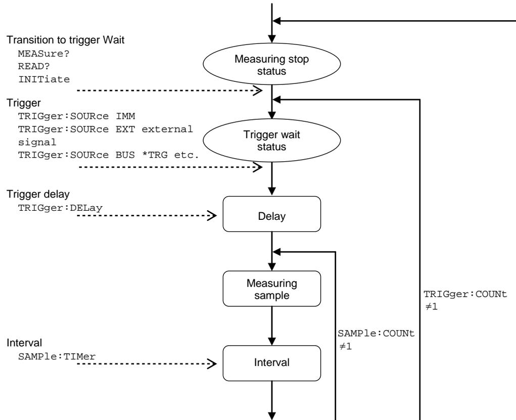
The REMOTE indicator of the annunciator cuts the measurement halt condition and besides in the above figure (The trigger waiting state and the measurement are operating) as follows and it changes.
