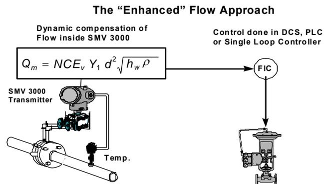
Figure 3 —Flow Compensation Using the “Enhanced” Approach
