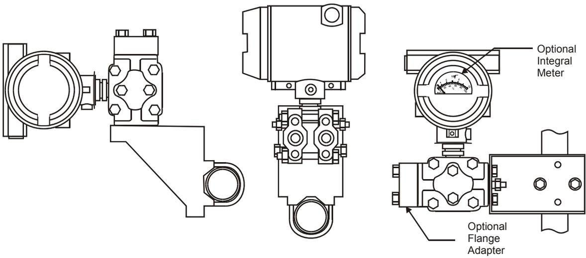
**Figure 9 —Examples of Typical Mounting Positions.**
