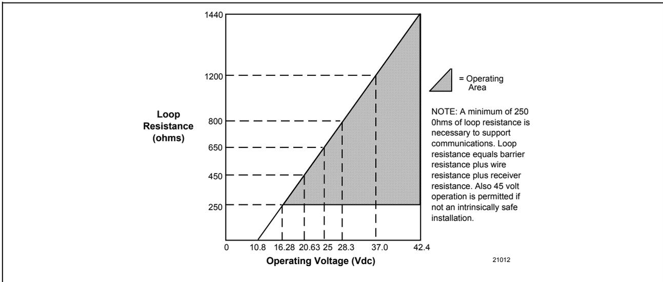
**Figure 7** —Supply Voltage and Loop Resistance Chart.
