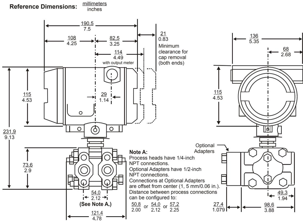
**Figure 8 —Approximate Mounting Dimensions for Reference Only.**
