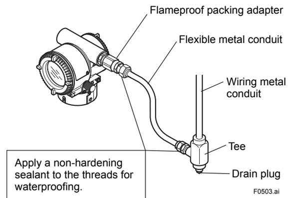
Figure 5.3 Typical Cable Wiring Using Flameproof Packing Adapter
