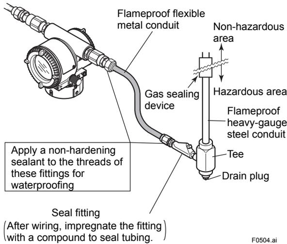
**Figure 5.4 Typical Wiring Using Flameproof Metal Conduit**
