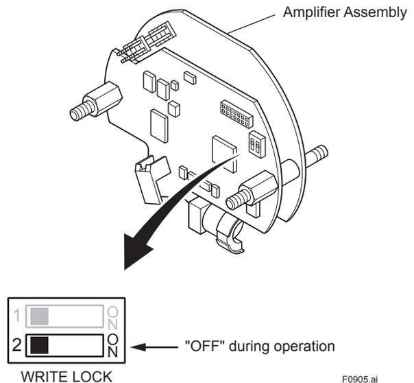
**Figure 9.5 WRITE\_LOCK Switch**
