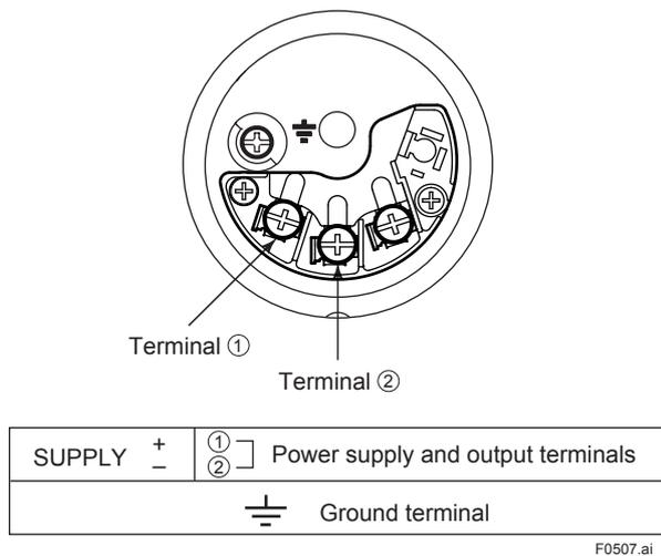
Figure 5.7 Wiring Diagram
