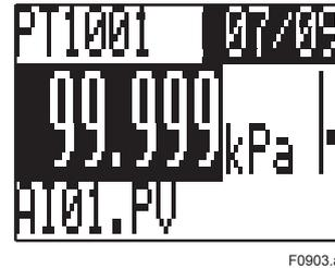
Figure 9.3 Example showing when process value have not correctly transferred
