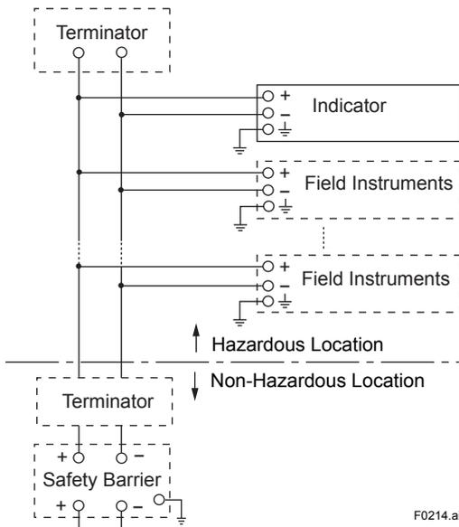
[Intrinsically safe apparatus level of protection "ic"]
