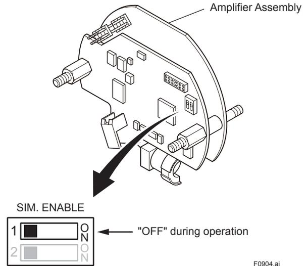
**Figure 9.4 SIMULATE\_ENABLE Switch**
