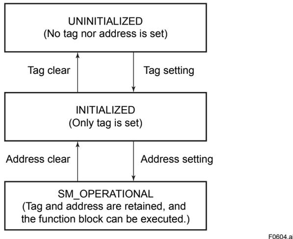
**Figure 6.4** Status Transition by Setting PD Tag and Node Address
