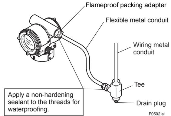
Figure 5.2 Typical Wiring Using Flexible Metal Conduit
