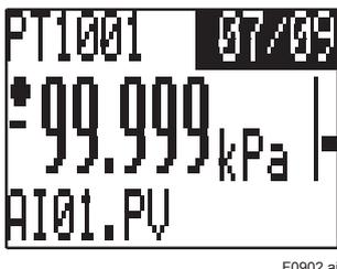
Figure 9.2 Example showing when process value have correctly transferred
