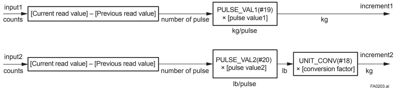
Figure A2.3 Increment Calculation with Counter Input
