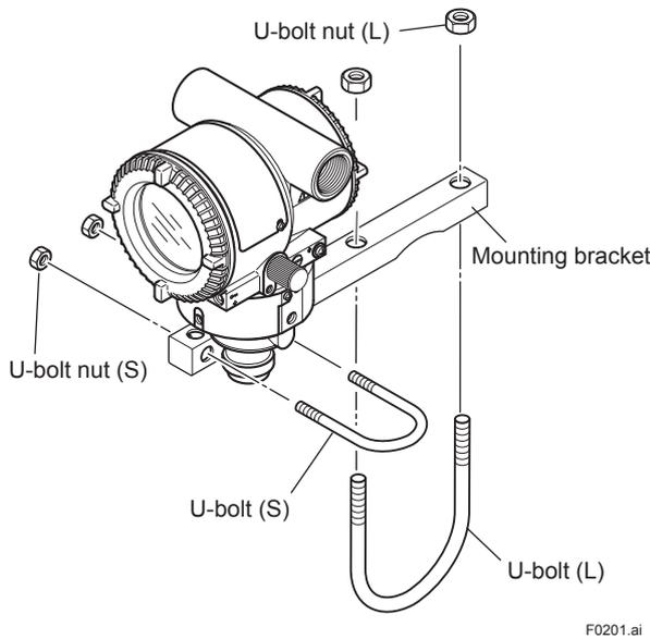
Figure 2.1 Indicator Mounting Hardware
