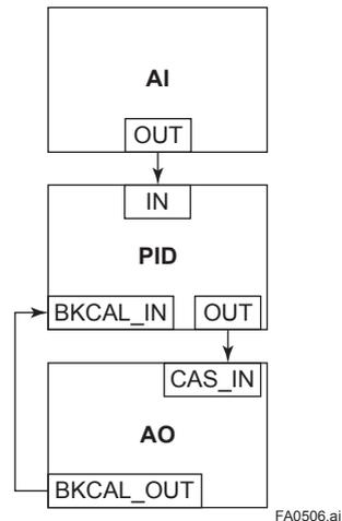
When configuring a simple PID control loop by combining an field device with a fieldbus valve positioner that contains an AO block, follow the procedure below to make the settings of the corresponding fieldbus function blocks:
