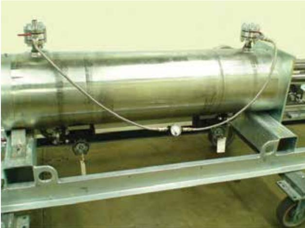
Figure 5-1: Static Leak Detection Set-up
