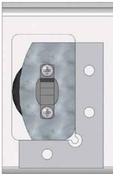
Figure 8-24: Correct Optical Switch Installation Bottom View
