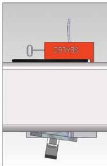
**Figure 8-27:** Improper Optical Switch Installation Bottom View 1
