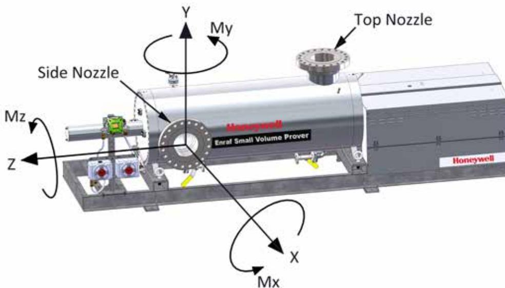
**Table 20:** Maximum allowable inlet and outlet flange loads
