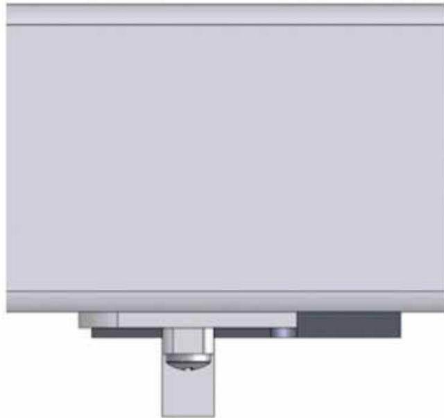
**Figure 8-25:** Correct Optical Switch Installation Side View
