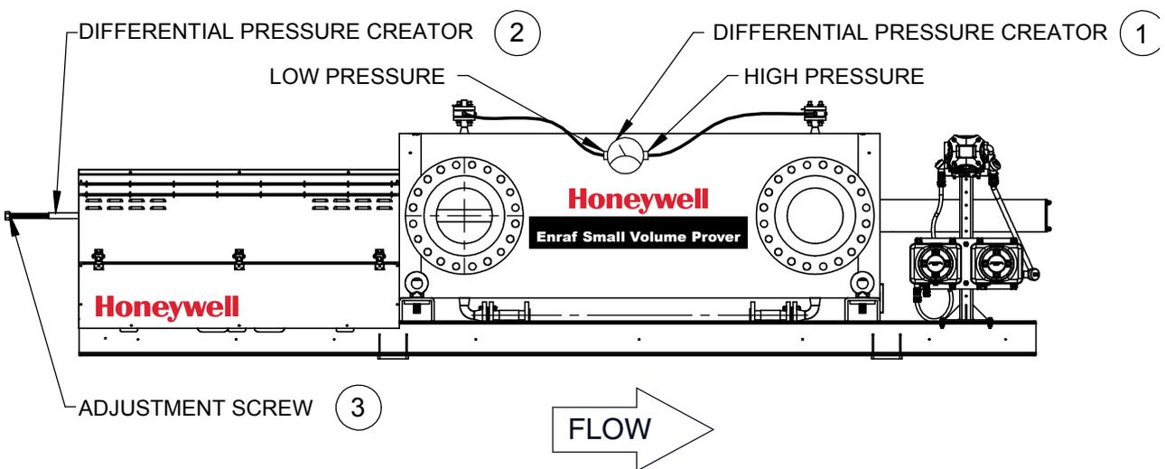
Figure 5-4: Static Leak Detection set-up overview
