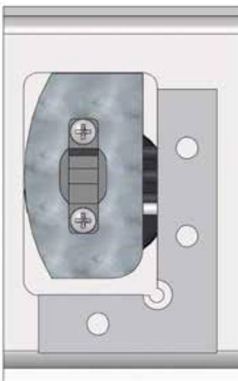
**Figure 8-26:** Improper Optical Switch Installation Side View
