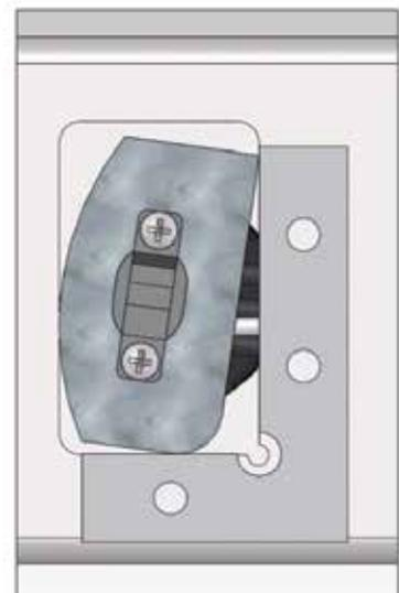
**Figure 8-28:** Improper Optical Switch Installation Bottom View 2
