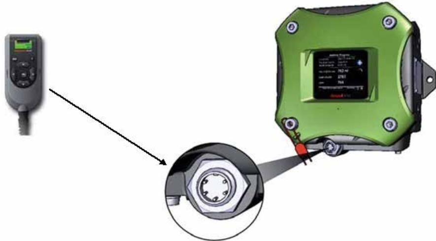
Figure 2-8: SVP Controller Box with LAD
