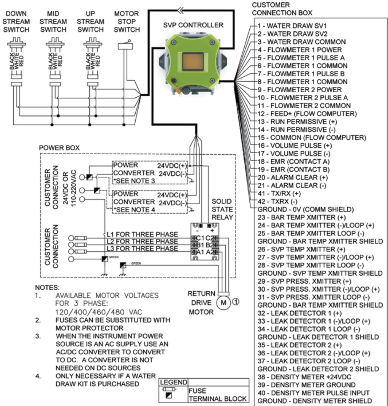
Figure 7-3: Wiring Diagram 3 Phase
