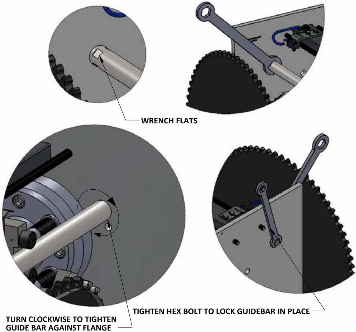
Figure 8-11: Tighten Guidebar
