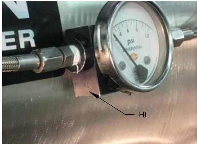
Figure 5-2: Gauge with HI & LOW markings
