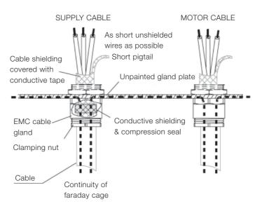
Figure 3-6 Essential points of power connections.
