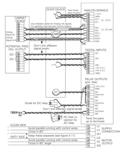
Figure 3-11 Principles of wiring inside CDM.
