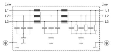
Figure 3-3 Example of filtering integrated in drive module.
