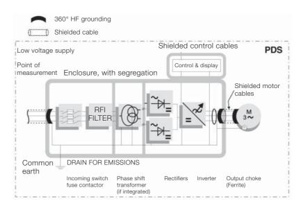
Note: All equipment inside must be enclosed Figure 4-4 12-pulse converter system fed at LV.
