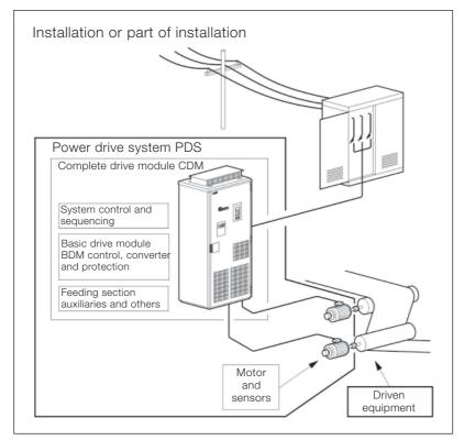
Figure 2-2 Abb reviations used in drives.
