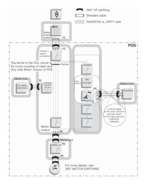
Figure 4-3 Basic scheme with by-pass.
