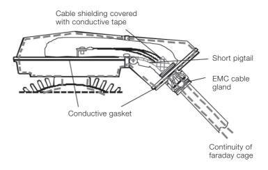
Figure 3-9 Essential points in motor cabling.
