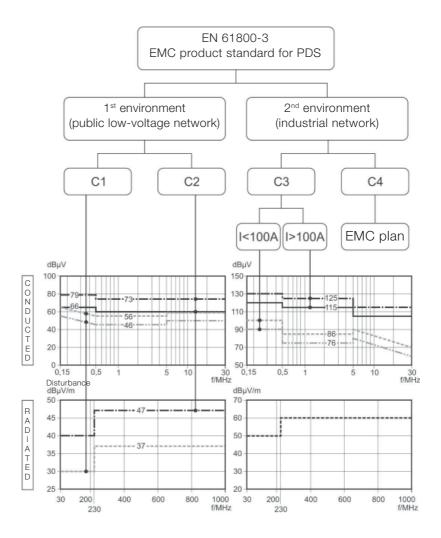
Figure 2-5 Emission limits for PDS.
