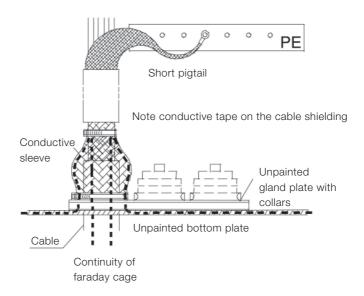
Figure 3-7 360° earthing with conductive sleeve.
