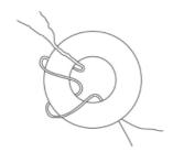
Figure 3-17 Ferrite ring in signal wire.
