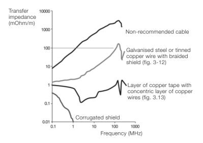
Figure 3-16 Transfer impedance for power cables.
