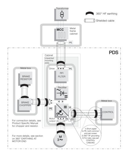
Figure 4-2 Typical PDS configuration.
