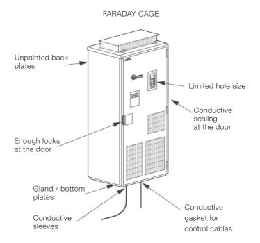
Figure 3-4 Typical enclosure aperture detail.
