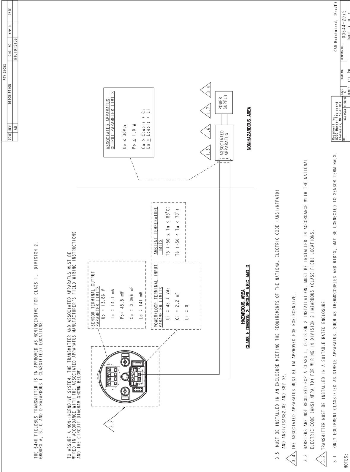
3.5 MUST BE INSTALLED IN AN ENCLOSURE MEETING THE REQUIREMENTS OF THE NATIONAL ELECTRIC CODE (ANSI/NFPA70) AND ANSI/ISA82.02 AND 82.03.
