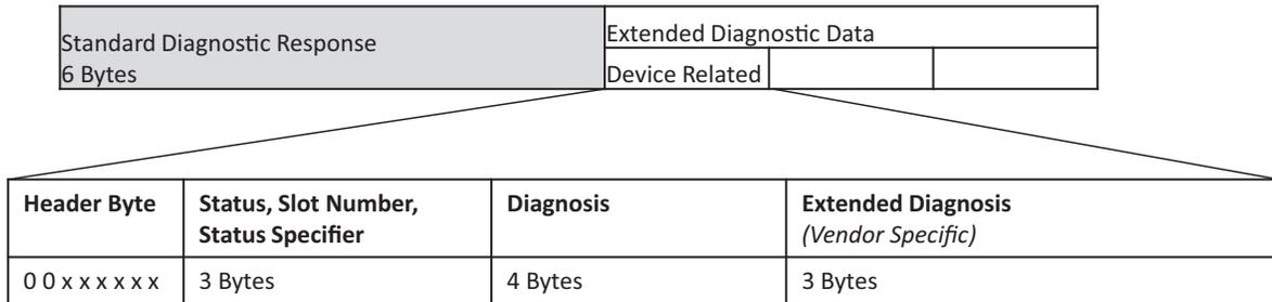
Figure 6-2. Diagnoses and Extended Diagnoses Bit Identification
