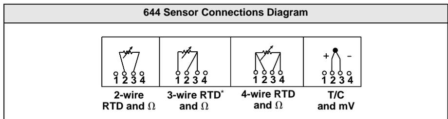
\* Emerson Process Management provides 4-wire sensors for all single element RTDs. Use these RTDs in 3-wire configurations by leaving the unneeded leads disconnected and insulated with electrical tape.
