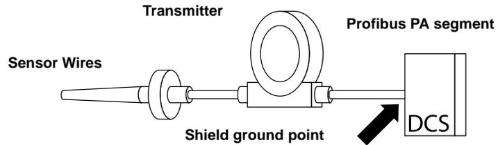
*Connect shields together, electrically isolated from the transmitter.*
