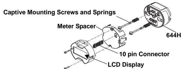
Use the following procedure to install the meter.
