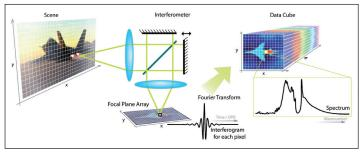
Schematized imaging Fourier transform spectroradiometer
