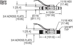
The SERIES P3 Flow Switches fit almost any piping requirements with compatible liquids. Choose the inlet and outlet port to be 3/8" male NPT or 1/4" male "Quick Disconnect" then select a quick disconnect acetal adapter for straight through flow or with a shut off valve
