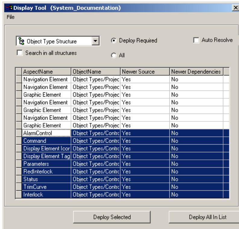
Figure 176. The Display Tool for deploying objects
