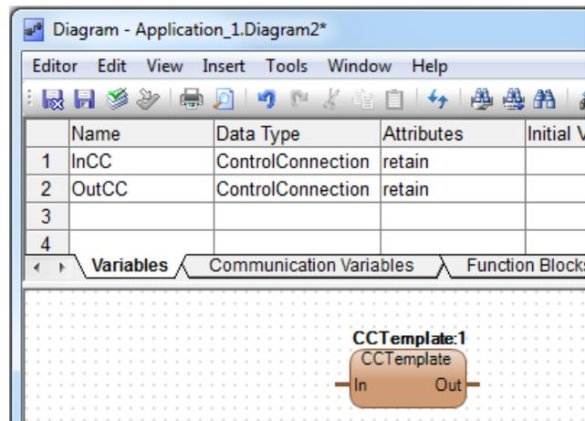
Figure 45. CCTemplate inserted in the graphical code block
