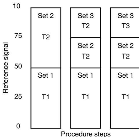
Figure 90. Example of the procedure for gain scheduling in three sets
