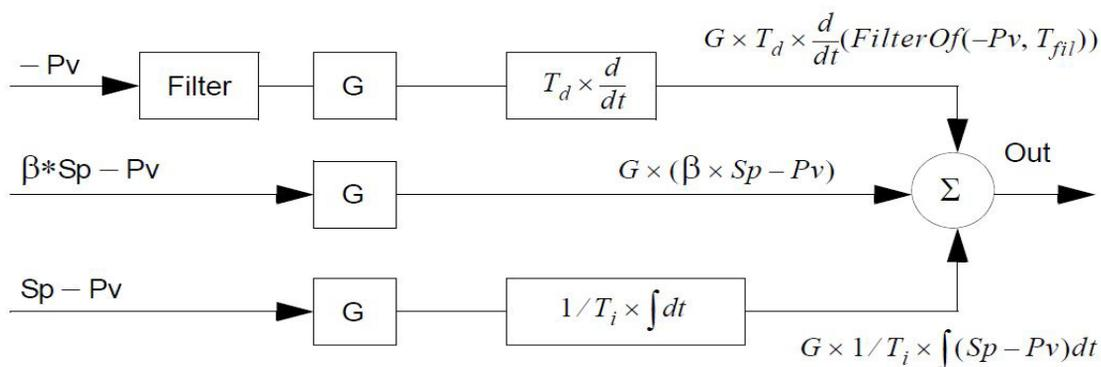
Figure 62. The principle of an ideal PID controller
