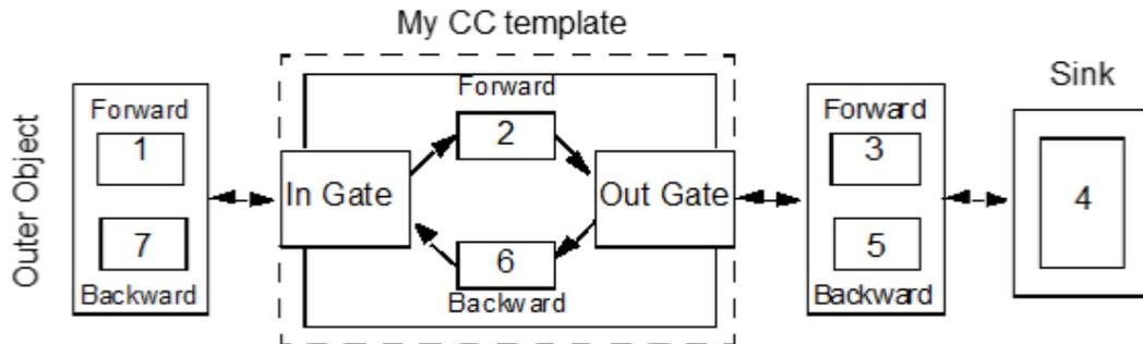
*Figure 30. My CC template object is protected by the Gate modules on both sides to ensure a secure signal traffic with ControlConnection*
