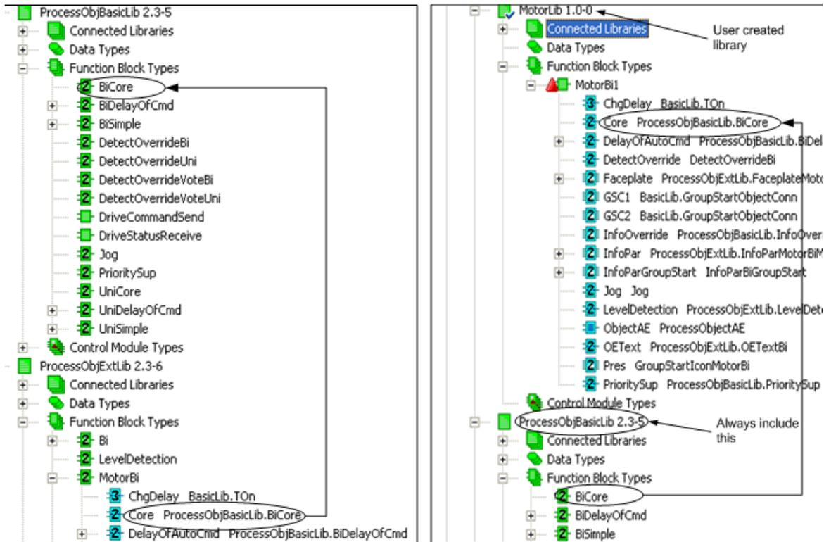
Figure 149. The core functionality in ProcessObjExtLib and in a user's self-defined library
