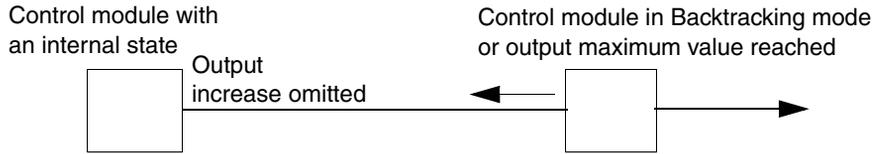
Figure 57. Example of when a succeeding control module has reached a limit value; the preceding control module stops further integration (anti-windup)
