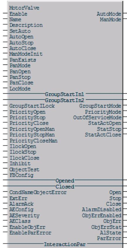
and is extended with alarm and interaction windows. The input interface is of type control connection that can be connected to an output object from a control loop.
