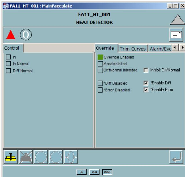
Figure 219. Parameter error indication in DetectorBool Faceplate
