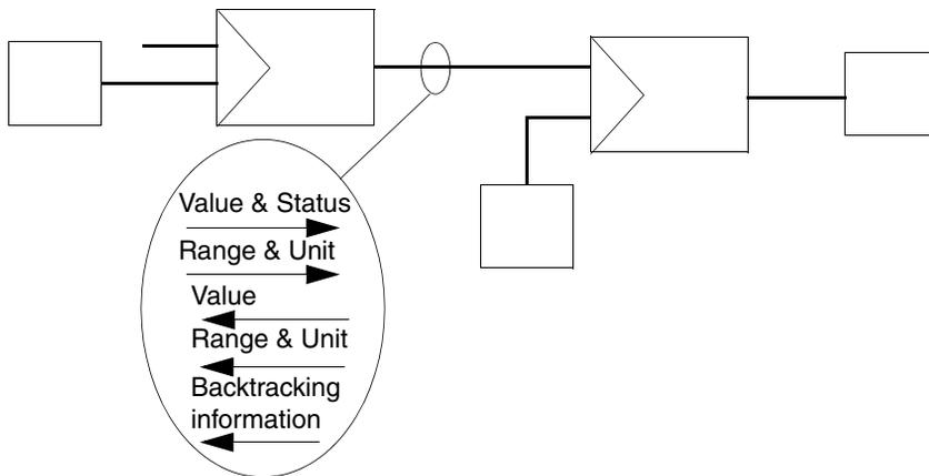
Figure 58. A graphical connection of ControlConnection type with its main signal flow forward and a flow backward
