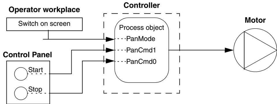
Figure 186. Control steps in Panel mode. This solution is recommended for large applications, where the *PanMode* parameter is connected to an operator workplace
