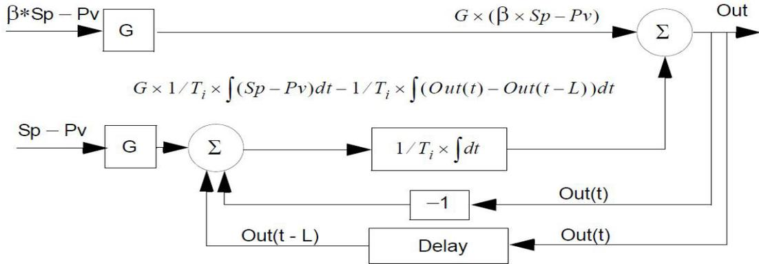
Figure 63. The principle of a PPI controller
