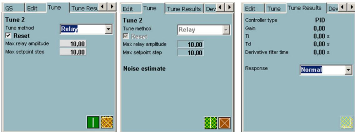
Figure 73. Autotuning in a PidAdvancedCC control module
