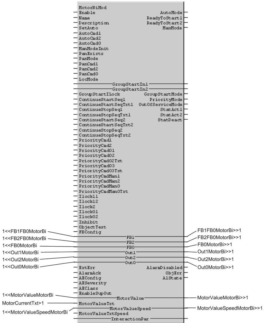
Figure 170. MotorBi function block with connections to variables
