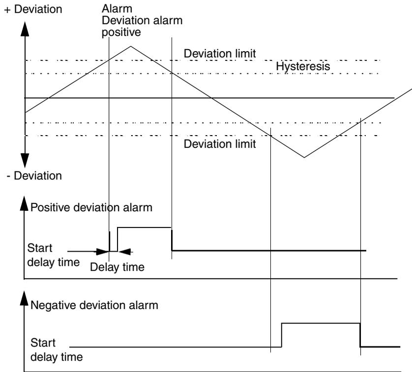
Figure 82. Overview of the controller deviation alarm limits
