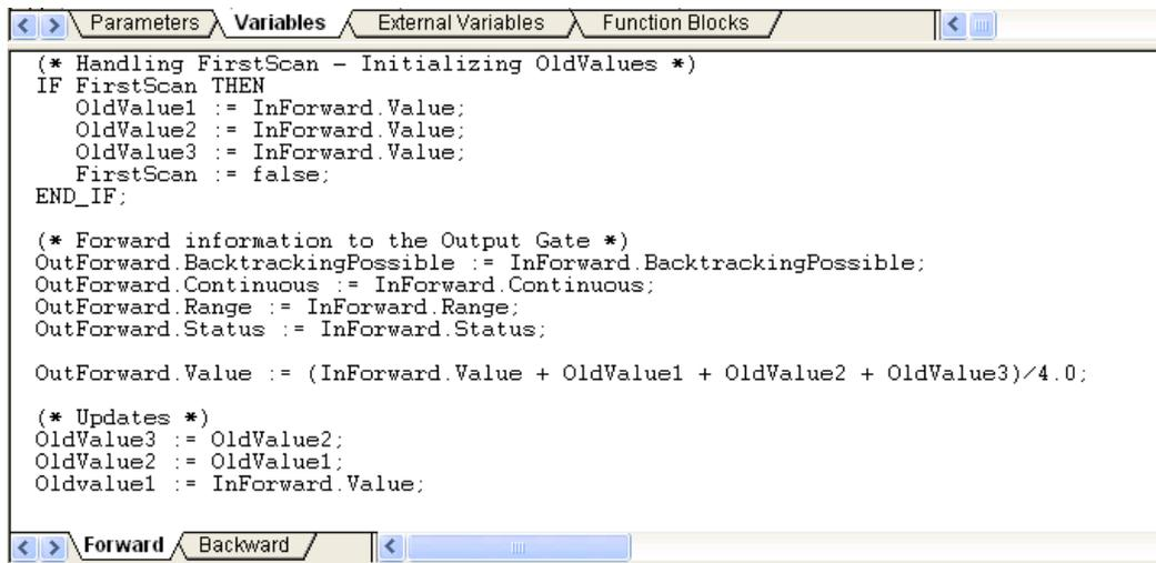
Figure 36. Programming code in the Forward code block
