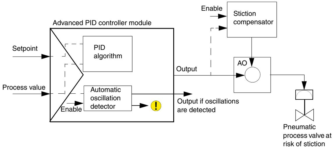
Figure 93. Principles for detecting and solving friction problems
