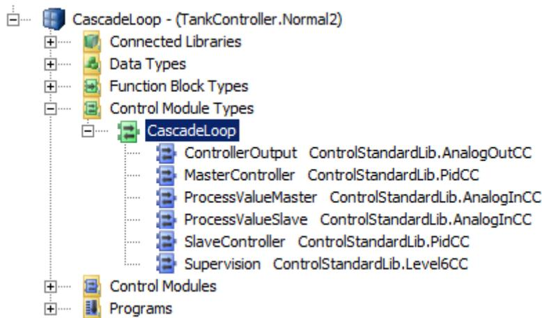
Figure 10. Cascade loop in Control Builder
