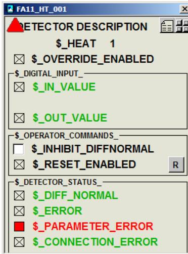
Figure 221. Parameter error indication in DetectorBool Interaction Window
