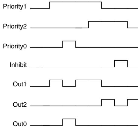
Figure 157. State diagram showing Priority command priorities and output signals with the effect of Inhibit
