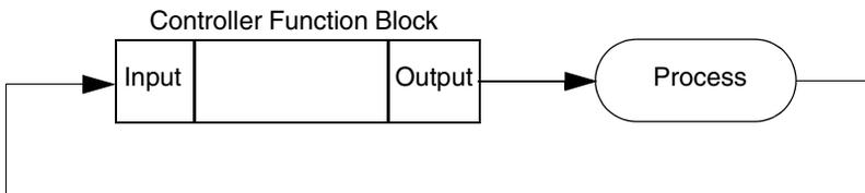
Figure 77. A control loop defined by a function block
