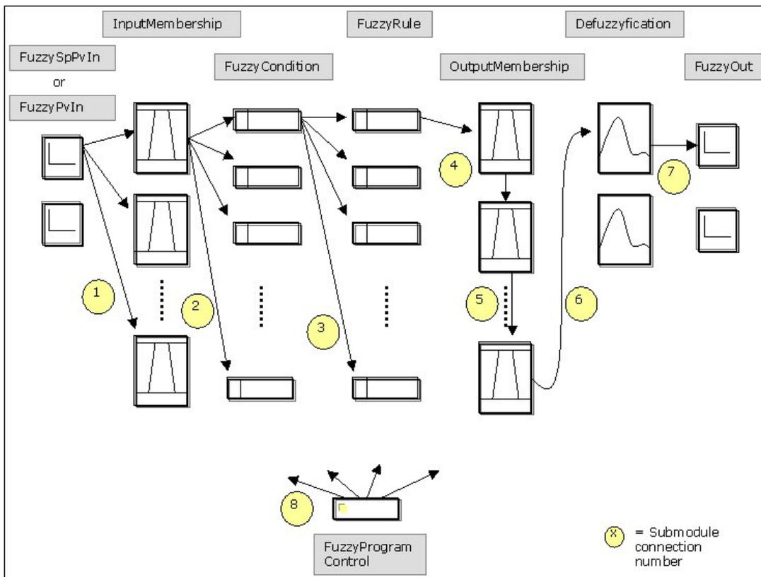
Figure 70. Sub-module connections in the fuzzy controller templates
