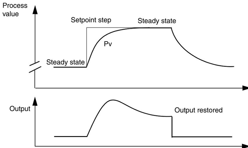
*Figure 86. Setpoint step identification and output restoration*
