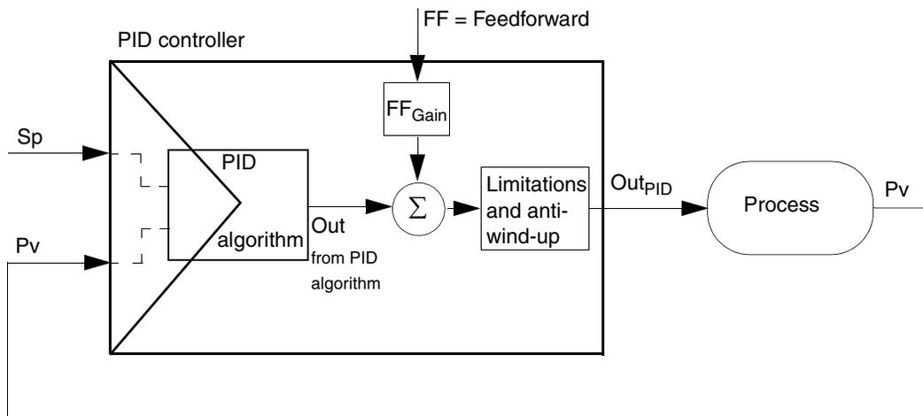
Figure 83. The feedforward principle in the controller
