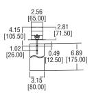
The MODEL AAFS Adjustable Air Flow Switch is capable of detecting a wide range of air velocities with minimal user calibration. Quality features include a stainless steel vane, galvanized steel base, and ABS enclosure.
